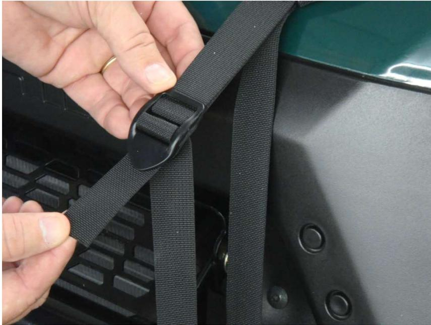
**Step 7:** Before tightening the hood straps, make sure the windshield/top is square and pulled tight from side to side. The holes in the hood panel should align with the hood mounts.
