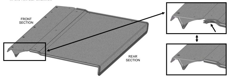
e) Install the roof to the vehicle using supplied hardware (Item G) as shown below and tighten. Note that some sections of the roll cage are hidden for better clarity.
