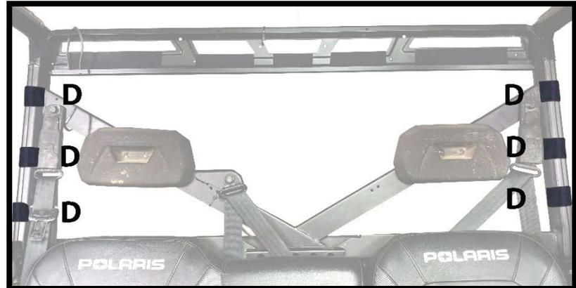
Figure 4: SHOWS PLACEMENT OF 6" VELCRO STRIPS (D).
