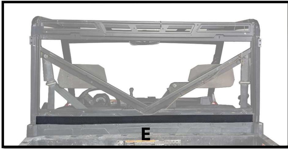
Figure 5: SHOWS PLACEMENT OF 54" VELCRO STRIP(E)
