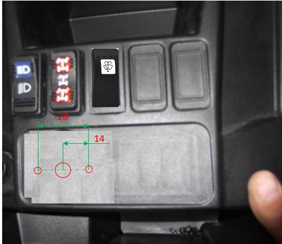
Lead the harness branches No.:1 and 2 from the heater to the UTV switch panel.
