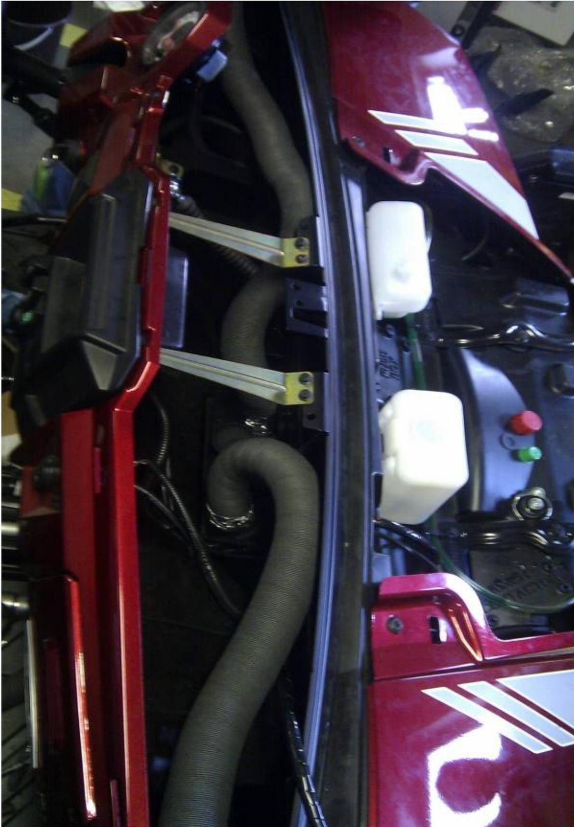
Uninstall the central tunnel cover from UTV's floor.
