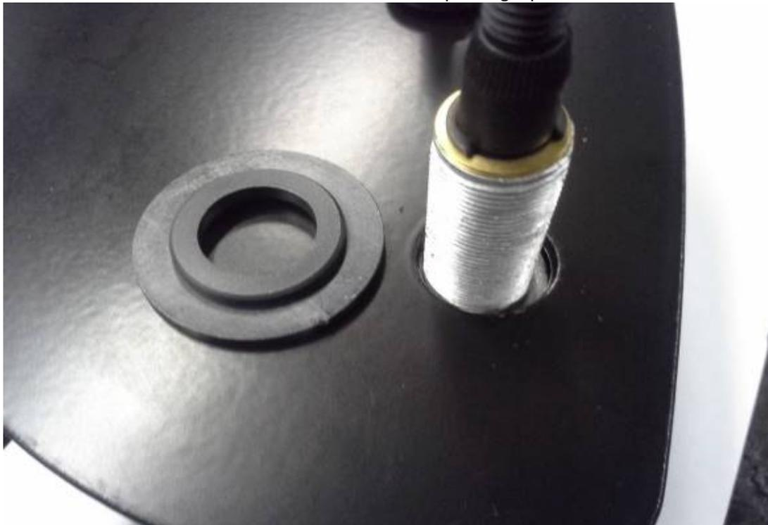
Place the washer onto shorter wiper pin.
