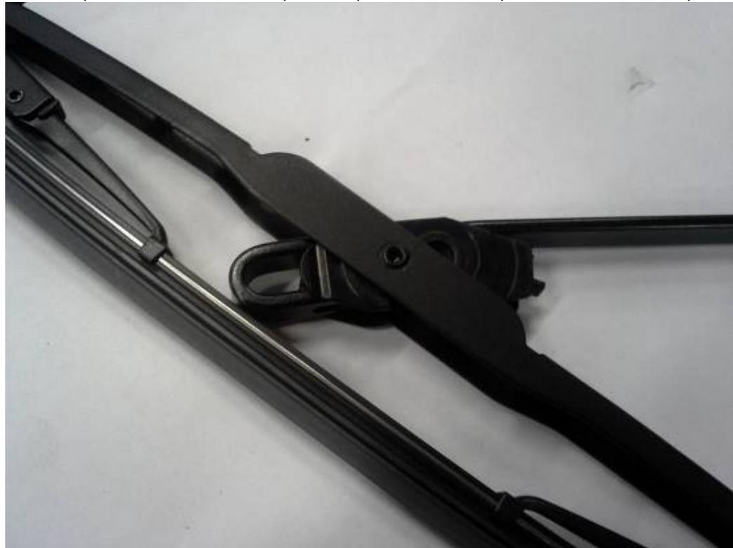
View onto installed wiper arm hook.
