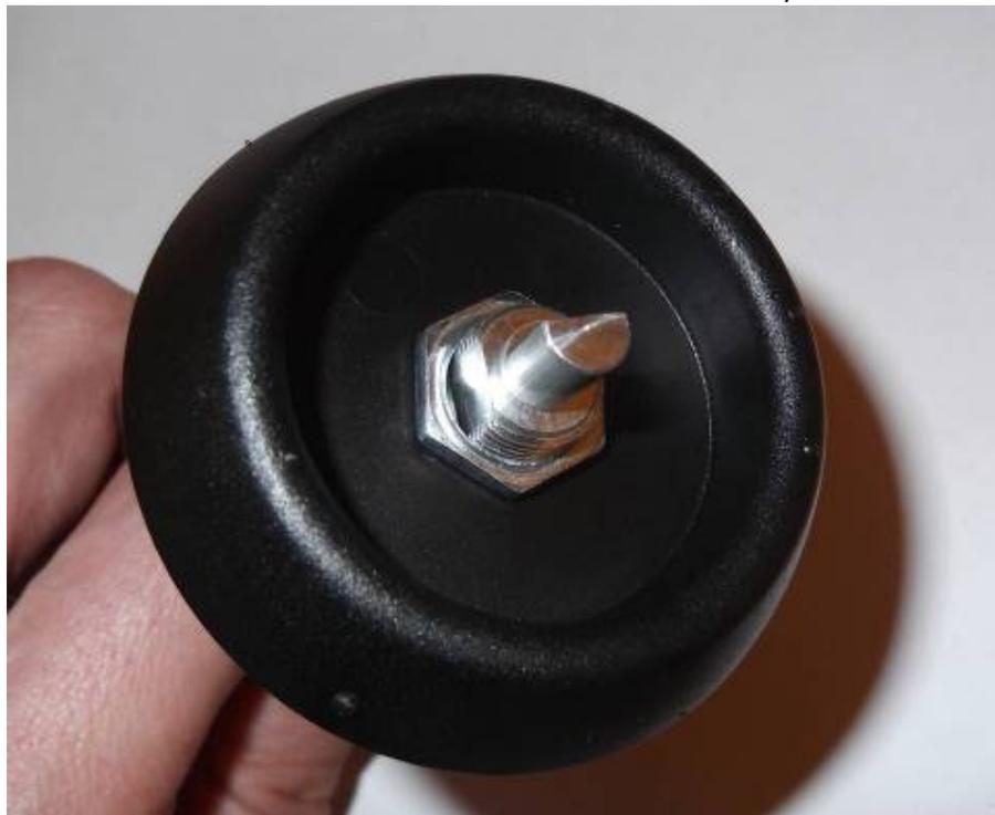
And place the plastic had onto the switch pin.
