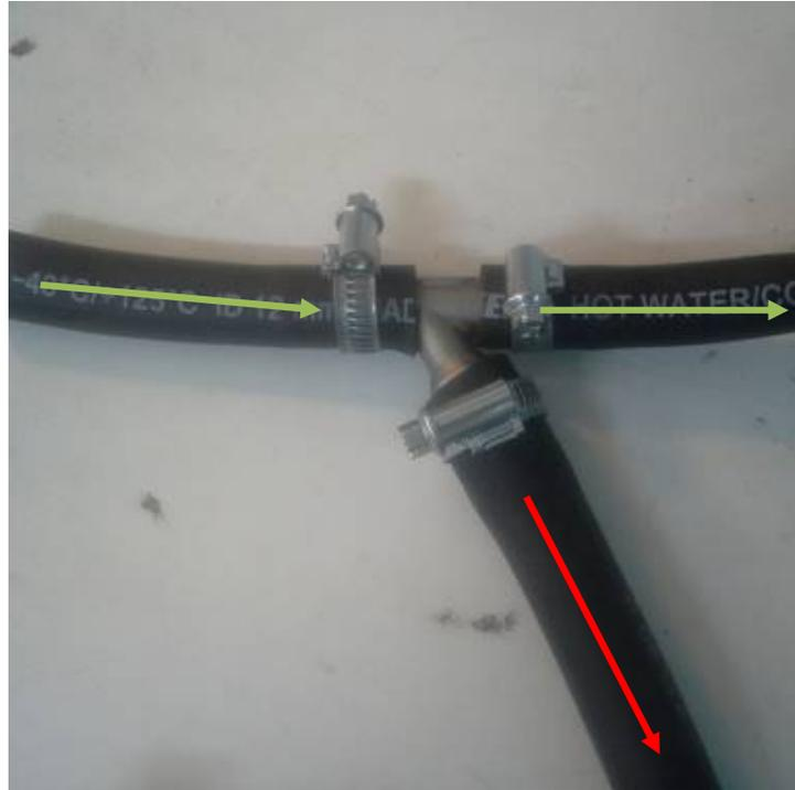
Lead the water hose (red arrow) through the floor tunnel.
