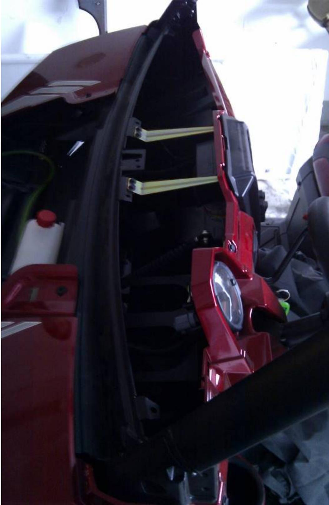
Take out the front dashboard cover and uninstall original screw (in red circle) from the UTV's plastic front wall and install the washer tank holder.
