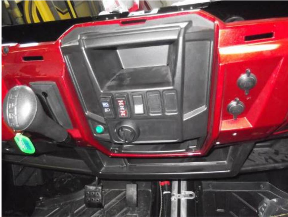
Take out the switch blind from the central panel. Pull the harness branch No.: 2 through the hole and connect the harness (red arrow) with the switch wiper/washer.
