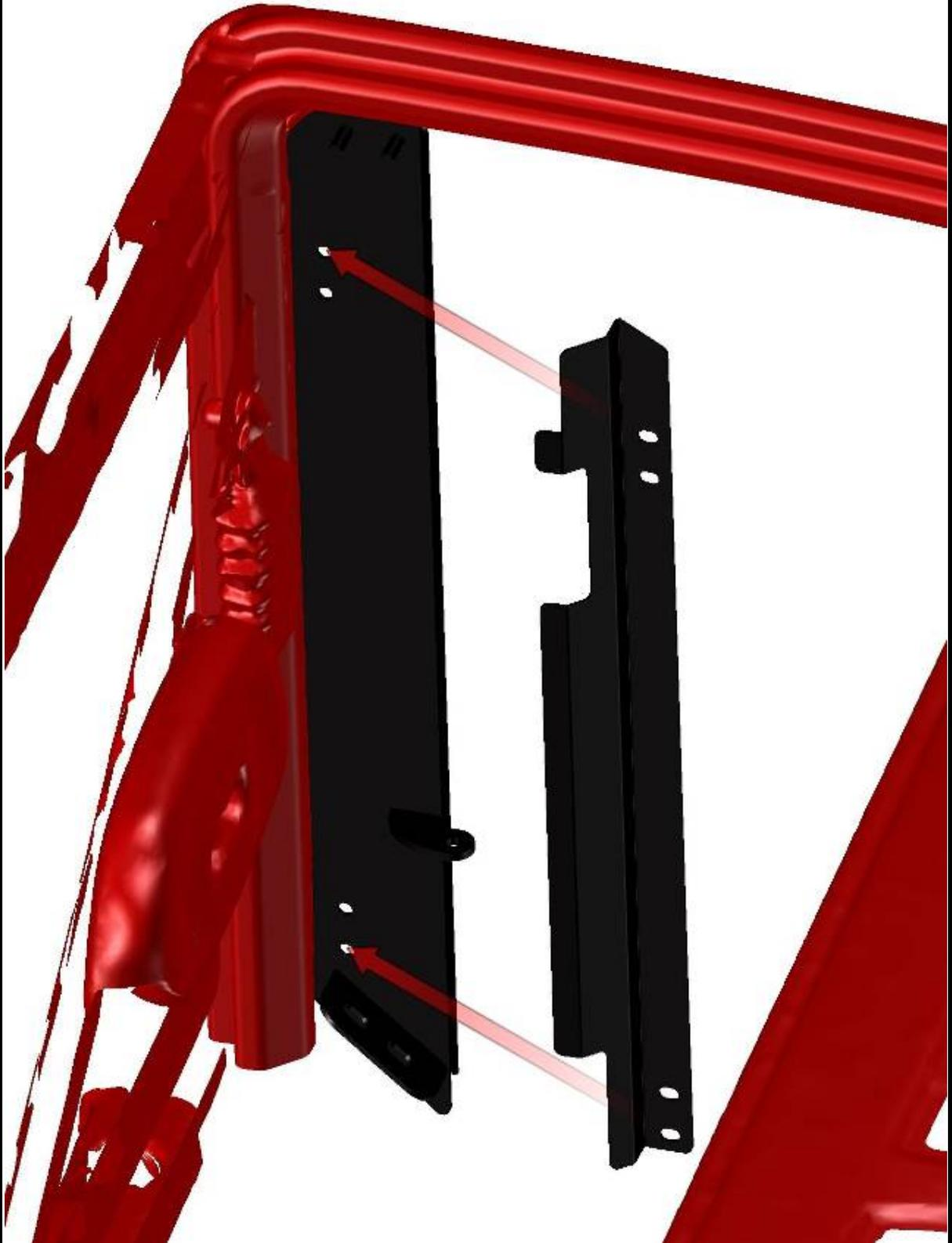
Place the correct hinges onto the door base.
