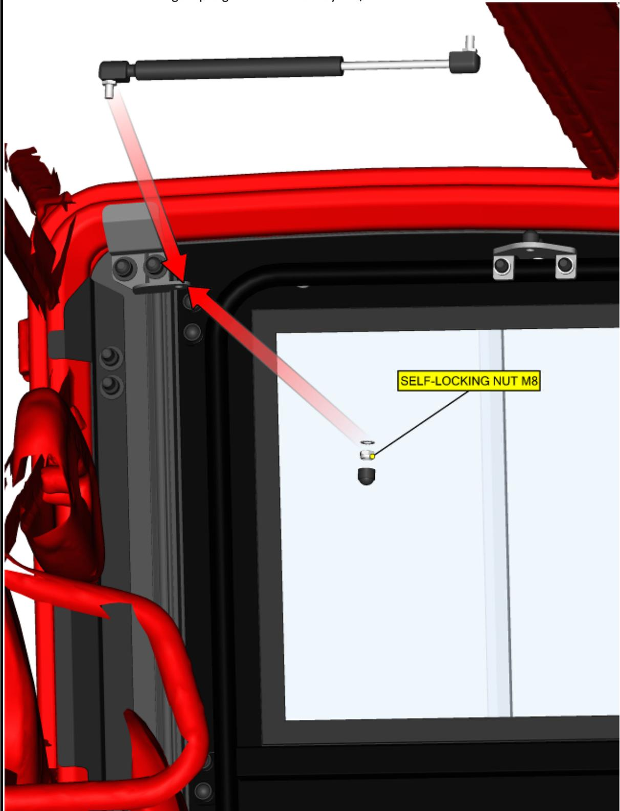
Install the gas spring holder onto the gas spring pin.
