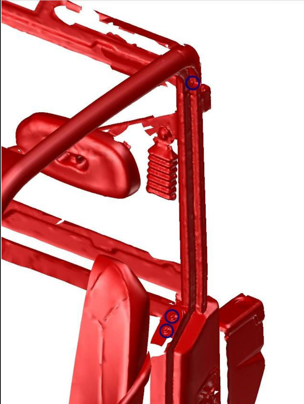
Place the left door base onto the roller cage and adjust that onto the best position.
