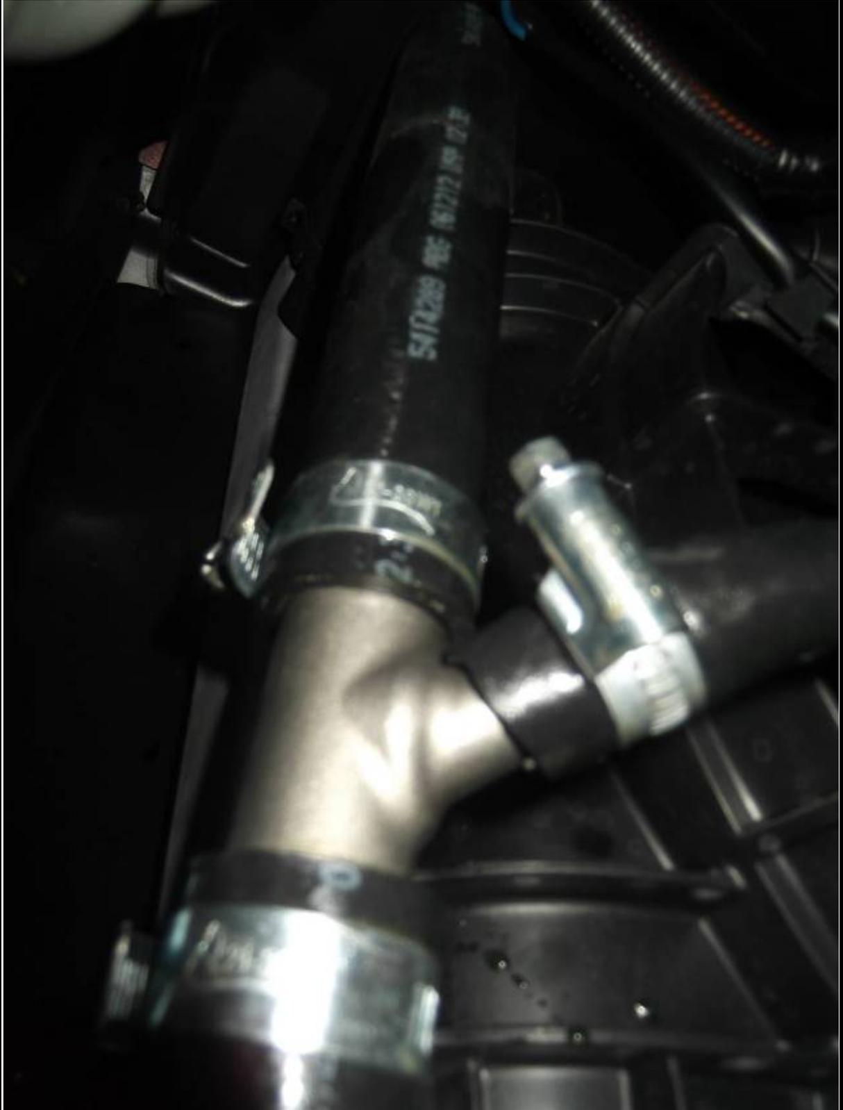
Cut the heater hose near "Y" coupling from previous page and insert the tightening straps. Install the air vent valve into the hose and fix these by straps. Tighten straps very hard.
