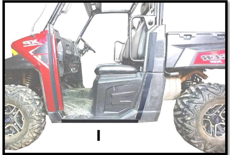
Figure 6: SHOWS PLACEMENT OF 29" VELCRO STRIP (I)
