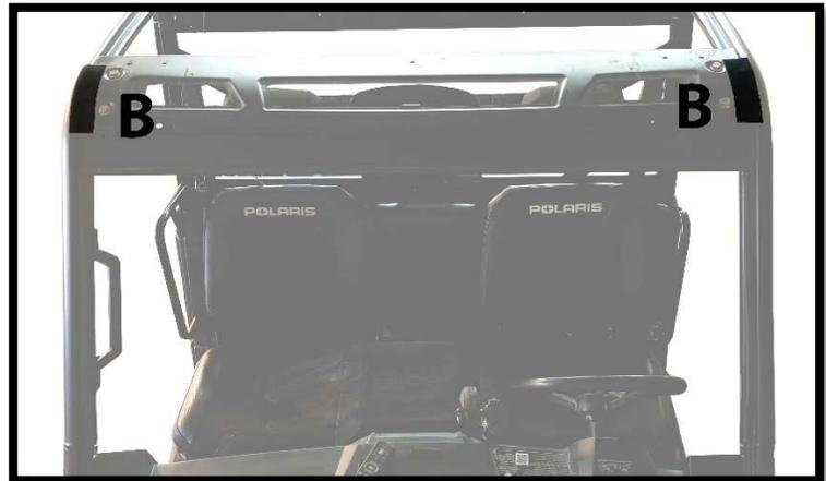
Figure 2: SHOWS PLACEMENT OF 6" VELCRO STRIPS (B)
