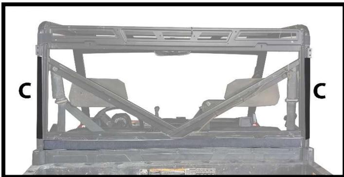
Figure 3: SHOWS PLACEMENT OF 18" VELCRO STRIPS (C)
