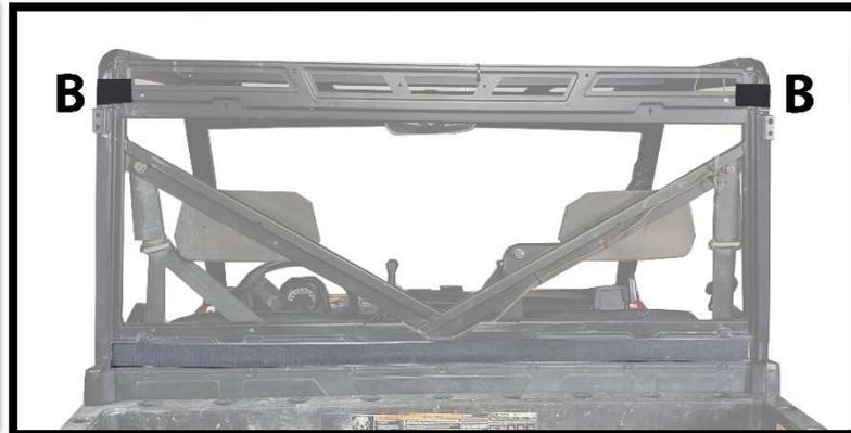
Figure 2: SHOWS PLACEMENT OF 6" VELCRO STRIPS (B).
