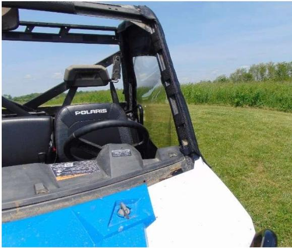
Figure 9: WHEN ATTACHING DOOR TO ADHESIVE VELCRO START WITH SIDE A. ALIGN BLACK TRIM ON THE DOOR PANEL TO THE EDGE OF THE INSET ROLL BAR. WRAP TABS AROUND THE INSIDE OF THE BAR AND ATTACH TO
