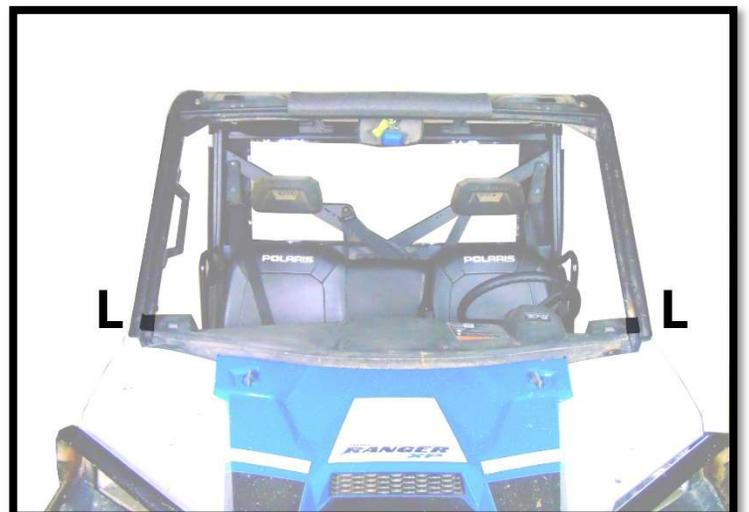
Figure 8: SHOWS PLACEMENT OF 3" VELCRO STRIPS. (L) FOR SMALL STRAP ON THE FRONT OF THE DOOR. PLACE TOWARD THE INTERIOR OF THE CAB NEXT TO DASH.
