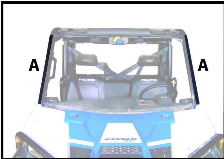
Figure 1: SHOWS PLACEMENT OF 26" VELCRO STRIPS (A) VELCRO STRAPS ON THE DOOR WILL WRAP AROUND ROLL-BAR AND CONNECT TO ADHESIVE VELCRO. You may move the straps around to avoid interference with other aftermarket products.
