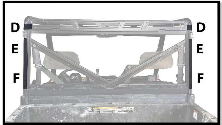
Figure 4: SHOWS PLACEMENT OF 4" AND 18" VELCRO STRIPS (D AND E) YOU CONNECT TABS E AND F TO THE 18" STRIP E.
