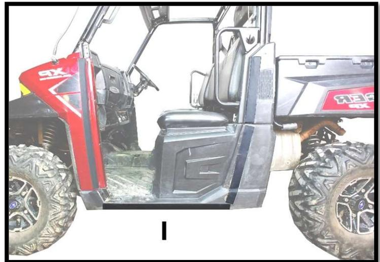
Figure 6: SHOWS PLACEMENT OF 29" VELCRO STRIP (I)
