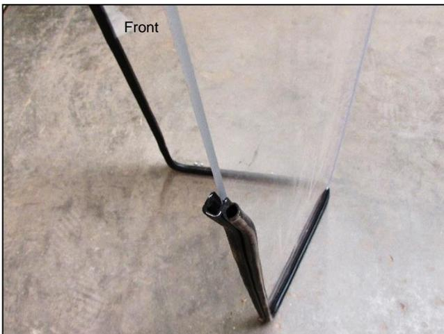
5. Press the channel of the gasket into the windshield. The bulb of the gasket should be facing the back of the windshield. It may help to use a rubber mallet to tap on the back of the gasket channel.
