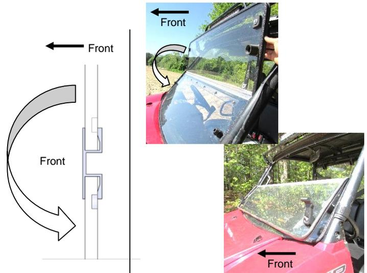
2. **NOTE: The orientation of gasket and parts are very important. See above.** The hinge will **ONLY** allow the windshield to fold down flat in one direction.
