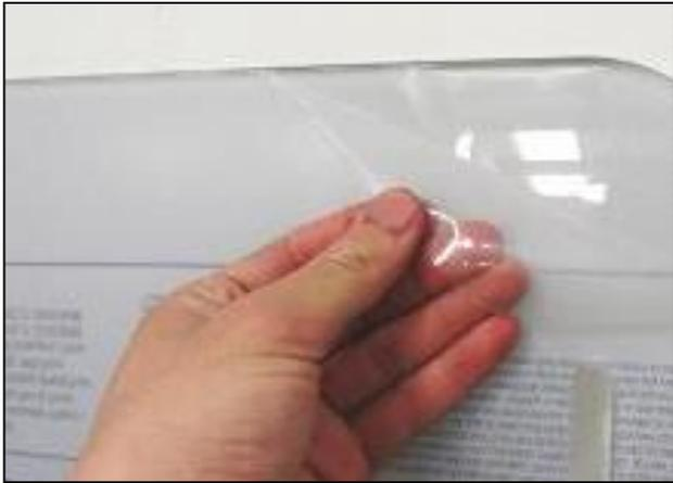
1. Peel the plastic fil back from all edges and holes of the windshield before beginning. Remove after windshield is fully installed.
