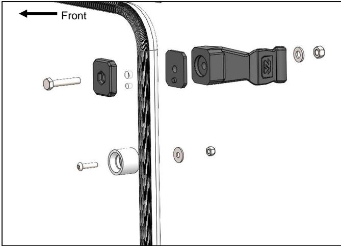
**7.** Attach the female rubber push plug in the single hole below the plastic lever. The plug should be on the **FRONT** of the windshield. If you have a full size, attach one in the center hole also.
