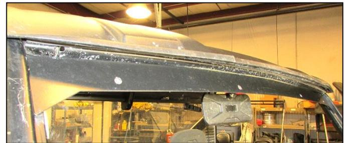
**10.** Place the header panel assembly on the windshield plane of the vehicle near the roof. The brackets should be facing the inside of the vehicle.
