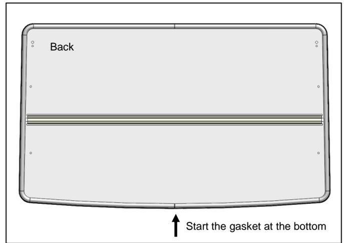
4. Attach the gasket with the bulb facing the **BACK** of the windshield. The gasket will seal between the windshield and the vehicle. Start the gasket at the middle of the bottom windshield.
