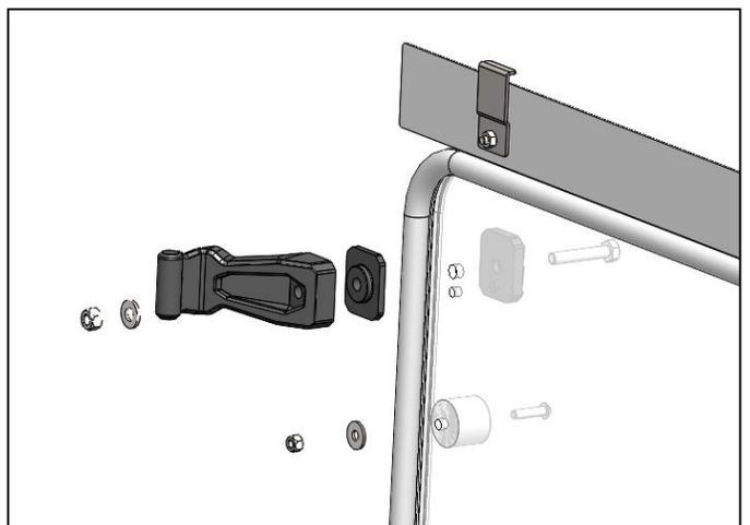
6. Attach the Lever using the inner and outer windshield mounting plates. The lever should be tight enough to just be able to turn with some force. The lever should be on **BACK** of the windshield. 1
