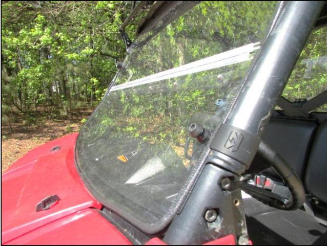
**13.** Place the windshield on the clamps and roll cage of the vehicle. Attach the male rubber plug and plastic spacer on the windshield in the order shown in the next step. It may be helpful to use a small object to push the bolt to the bottom of the plug.
