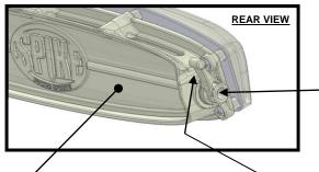
As shown on the rear-view image, the <u>lever</u> is installed by default on the right side of the vent.
