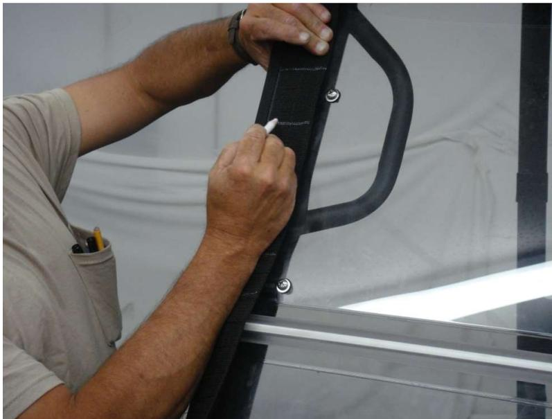
**Step 8:** Cut the webbing strip with household scissors. **AGAIN, DO NOT CUT INTO THE BINDING.** Seal the frayed edges with a lighter. Have a wet cloth handy to dab the edges if needed.
