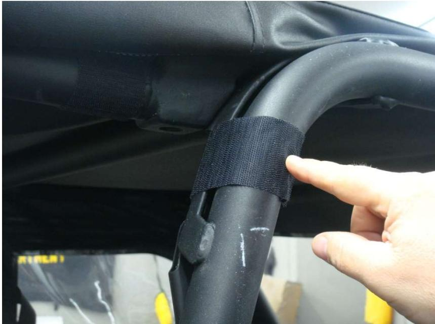
Reference A, B, and C-wrap adhesive hook strips horizontally around roll bars.
