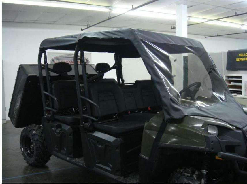
**Step 4:** Pull the enclosure (each side of the front windshield) downward toward the front of the vehicle and attach the 8" and 6" webbing/loop tabs to the corresponding adhesive hook strips on the front roll bar uprights. Reposition the webbing/loop tabs to square the windshield to the cab frame.
