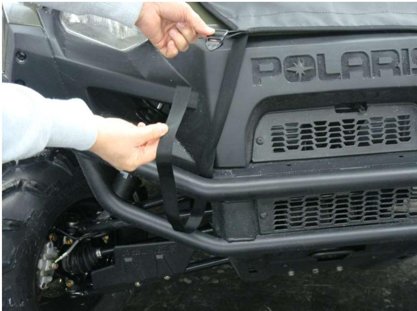
Figure 5.1 – guide front Hood straps around bumper
