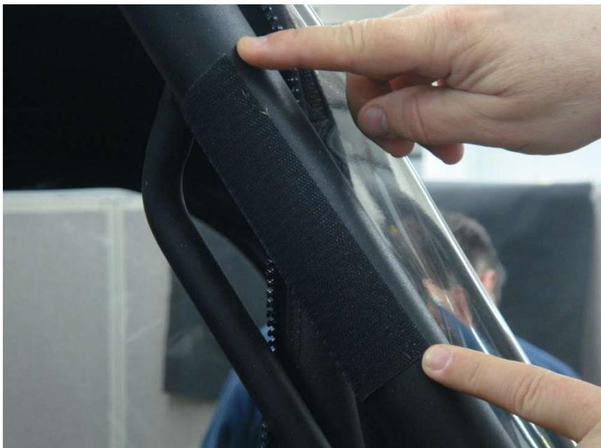
Reference D & E-Install adhesive hook strips vertically along the outside edge of the front roll bar uprights.
