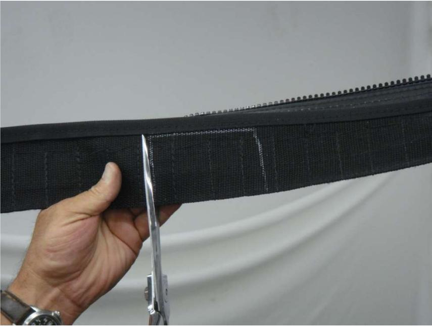
Figure 8.3 – Cut the Tab being very careful not to cut the binding at the edge
