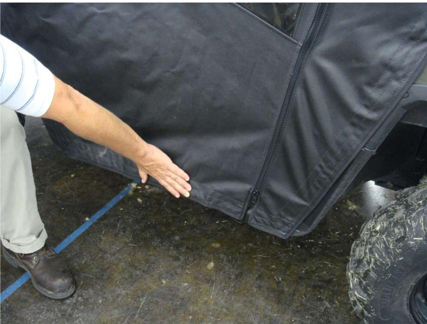
Figure 9.2 – attach Door Rocker Panel Enclosure 28" Velcro Tabs
