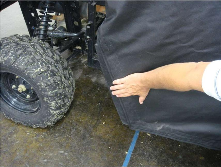
Figure 9.1 – attach Door Rear Panel Enclosure 18 ½" Velcro Tabs
