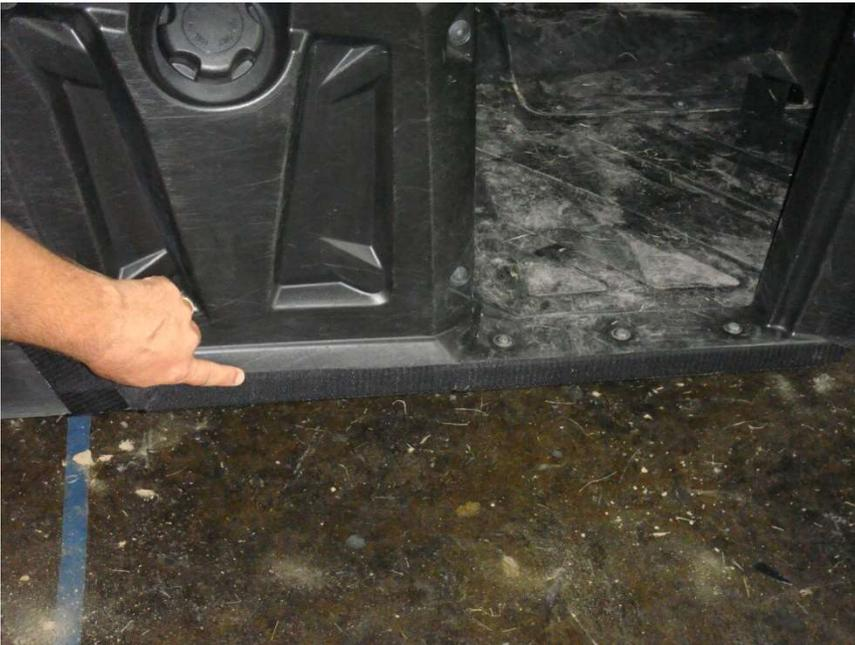
Figure 5.1 – attach 28” Velcro Strips horizontally along the door Rocker Panel – align the top side and fold the bottom 1” underneath the Rocker Panel
