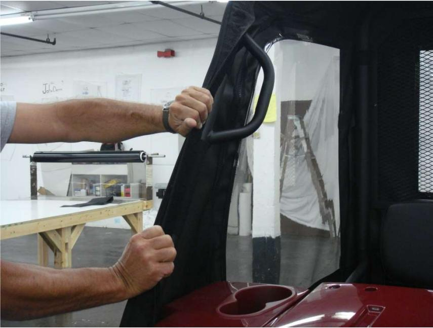
Figure 8.1 – attach Windshield Roll Bar post Velcro Tabs to installed 28” and 9” Velcro Strips
