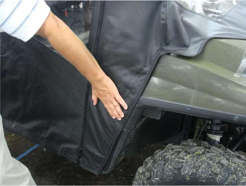
Figure 9.3 – attach Door Front Cowl Panel Enclosure 24 ½” Velcro Tabs
