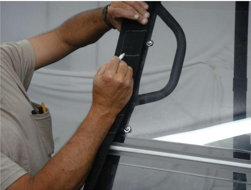
Figure 8.2 - Mark windshield tabs where hard windshield clamps are located along the windshield Roll Bar
