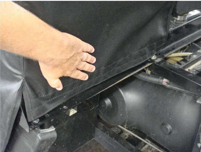
Figure 7.1 - square rear of enclosure to cab and attach rear enclosure Velcro tab to installed Velcro strips
