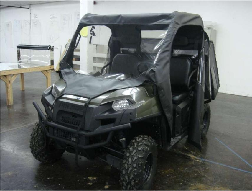
Figure 6.1 - place enclosure on vehicle cab roll bar structure – align enclosure seams with center of roll bars
