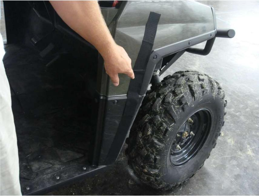
Figure 4.1 – attach 24 ½” Velcro Strips vertically along the Front Cowl Panel
