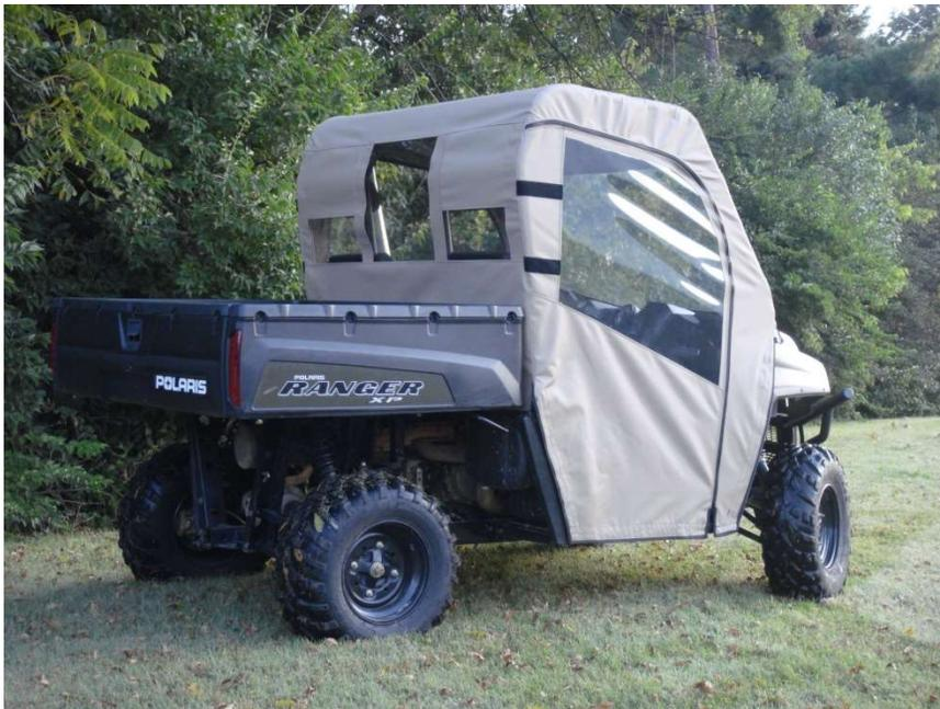
Figure 10.1 – Repeat Steps 8 and 9 until the enclosure fits snugly to the vehicle roll bar cab
