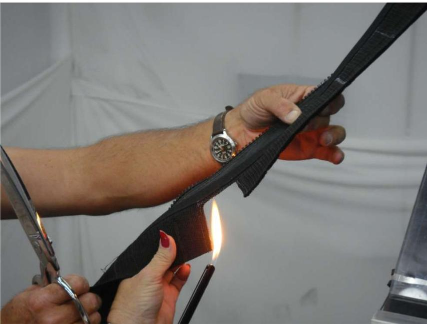
Figure 8.4 – Seal Frayed Tab thread at the cut area using a lighter
