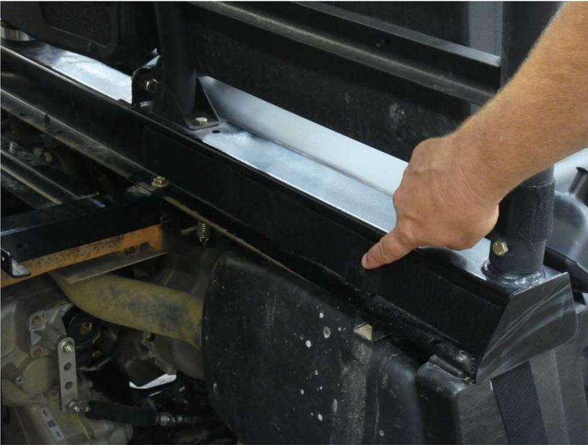
Figure 2.1 – attach 21" and 17" Velcro strips to the Rear Cab Frame
