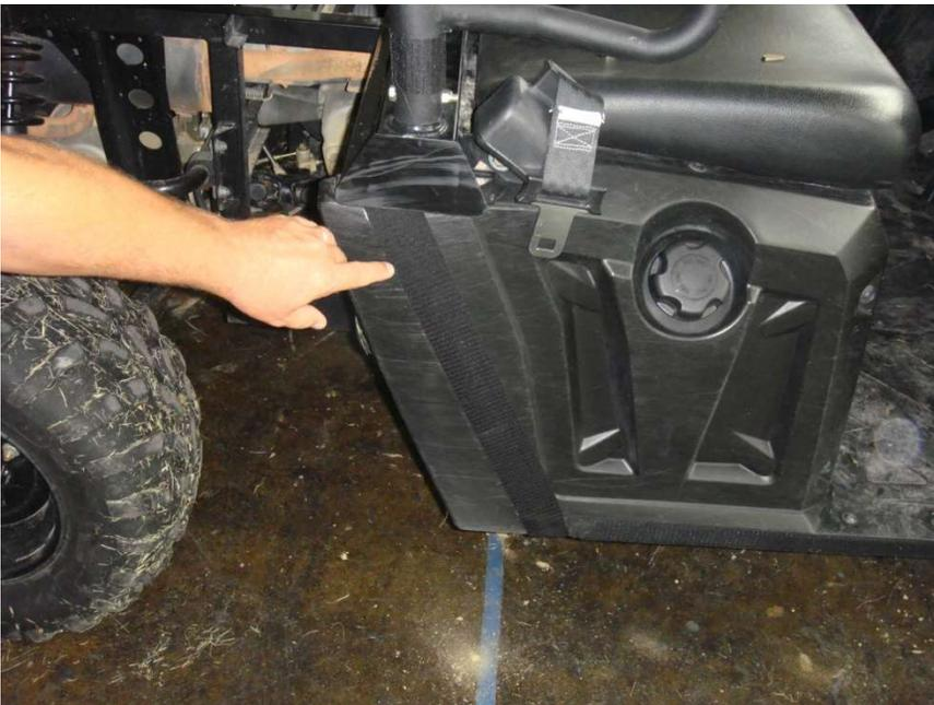
Figure 3.1 - attach 18 ½” Velcro Strips vertically along the Rear Door Panel
