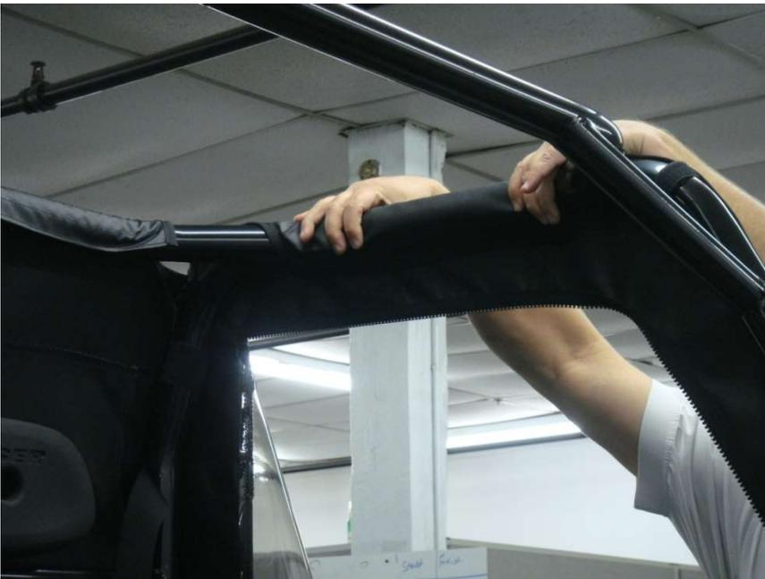
Figure 9.3 – attach 15" Door Top Roll Bar Frame Velcro Tabs
