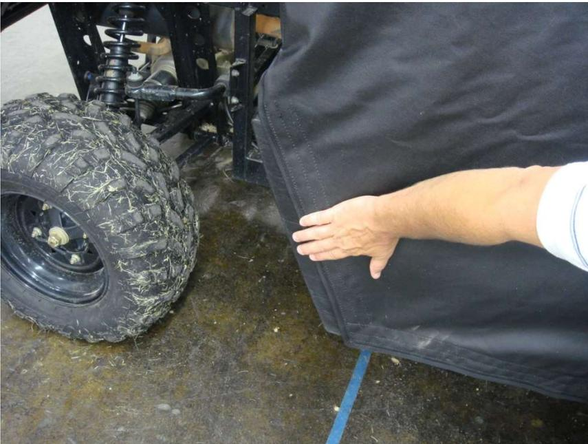
Figure 11.1 – attach Door Rear Panel Enclosure 18 ½" and 4 ½" Velcro Tabs
