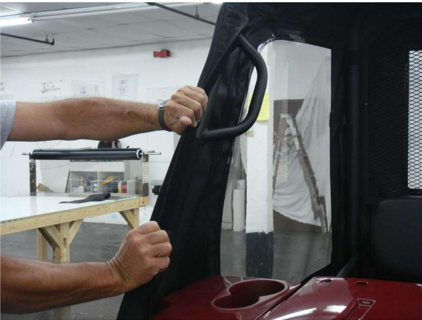
Figure 10.1 – attach Windshield Roll Bar post Velcro Tabs to installed 28” and 9” Velcro Strips
