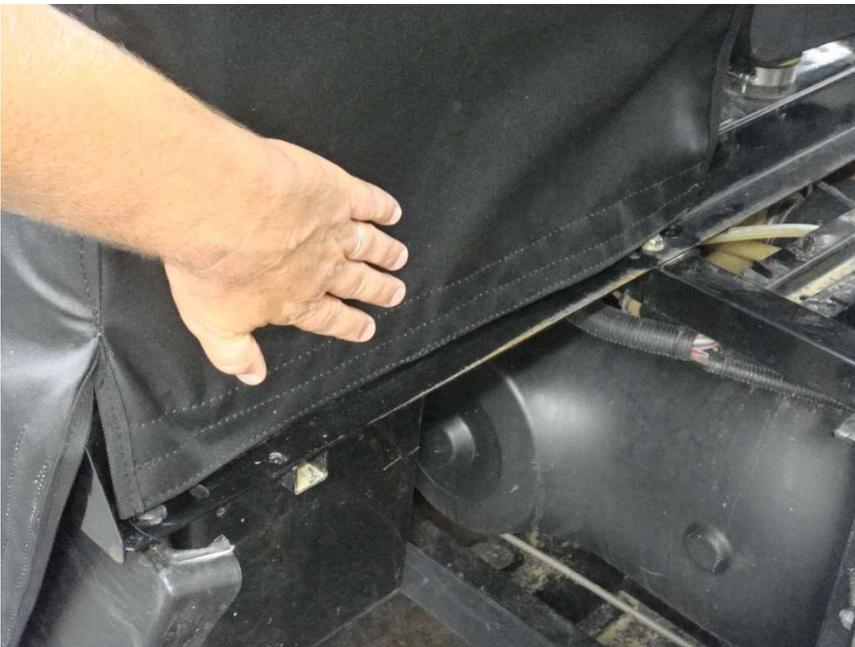
Figure 9.1 - square rear of enclosure to cab and attach rear enclosure Velcro tab to installed Velcro strips
