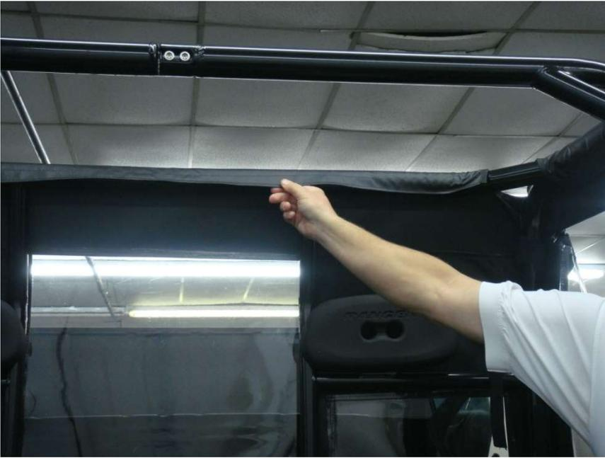
Figure 9.4 – attach 49” Rear Top Roll Bar Frame Velcro Tabs
