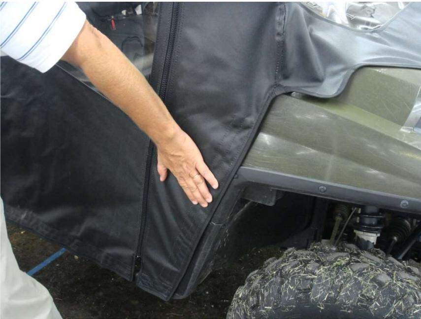
Figure 11.3 – attach Door Front Cowl Panel Enclosure 24 ½" Velcro Tabs
