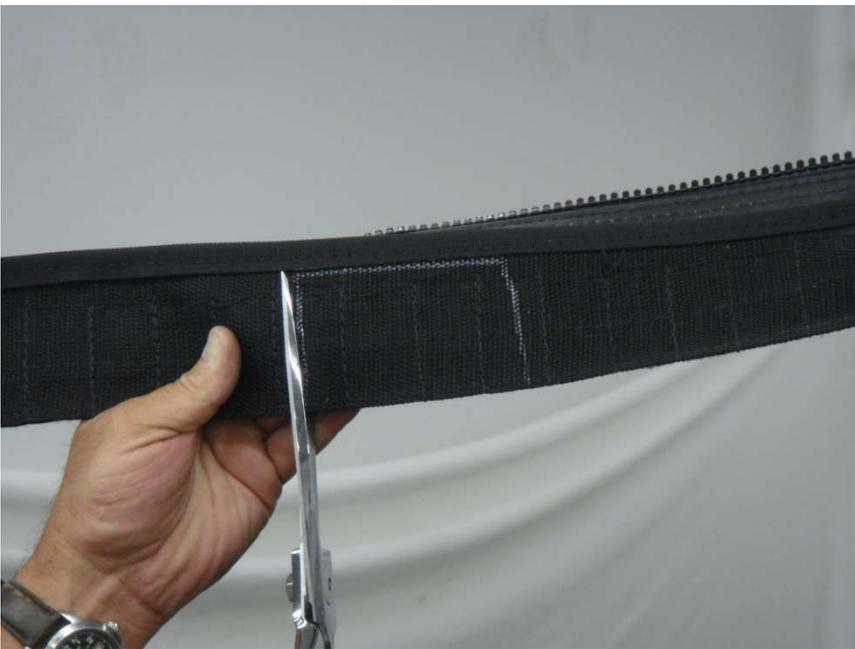
Figure 10.3 – Cut the Tab being very careful not to cut the binding at the edge
