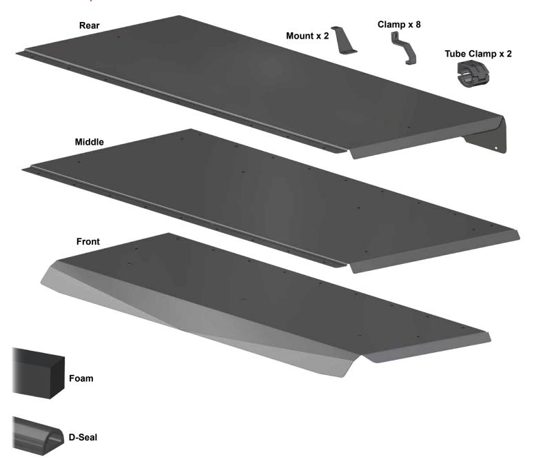
When installing components, do not tighten any hardware completely unless noted.
