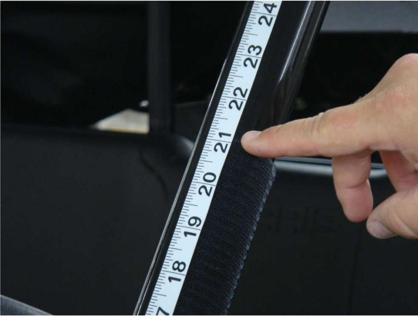
Figure 3.2 - attach 10" Velcro strips vertically approx 21" above the front roll bar post cowl opening
