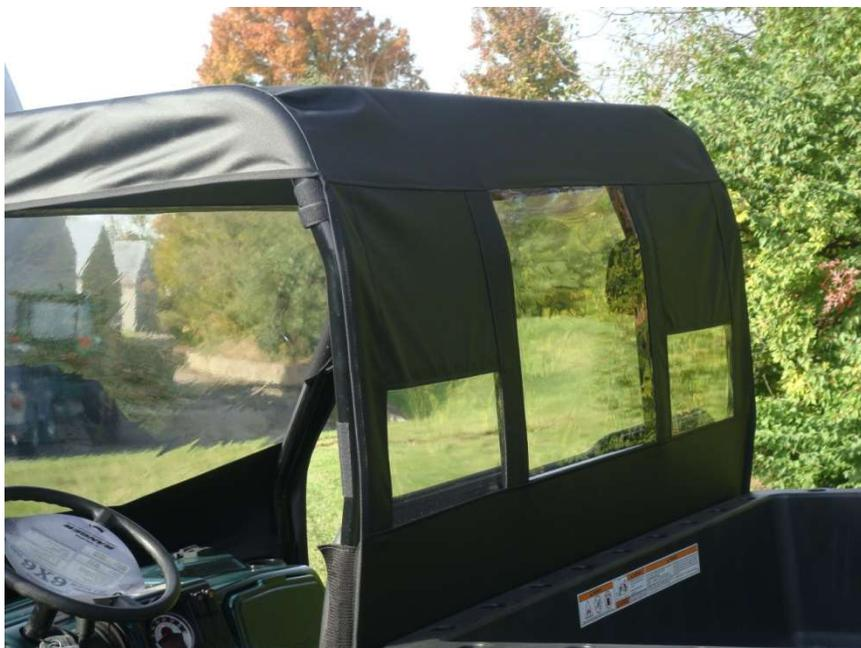
Figure 9.2 – Rear windows should be tight across the back of the Cab
