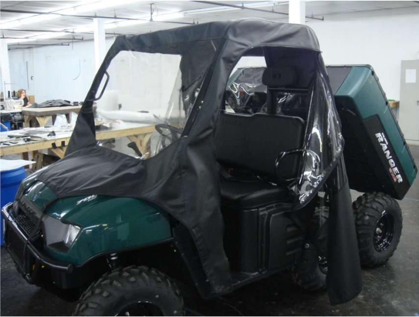
Figure 4.1 - place enclosure on vehicle cab roll bar structure – align enclosure seams with center of roll bars
