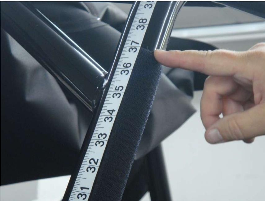
Figure 3.3 - attach 10" Velcro Strips vertically approx 37" above the front roll bar post cowl opening
