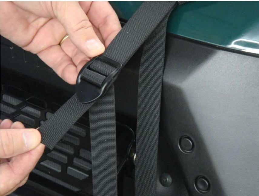
Figure 6.2 - thread front hood straps through the buckles
