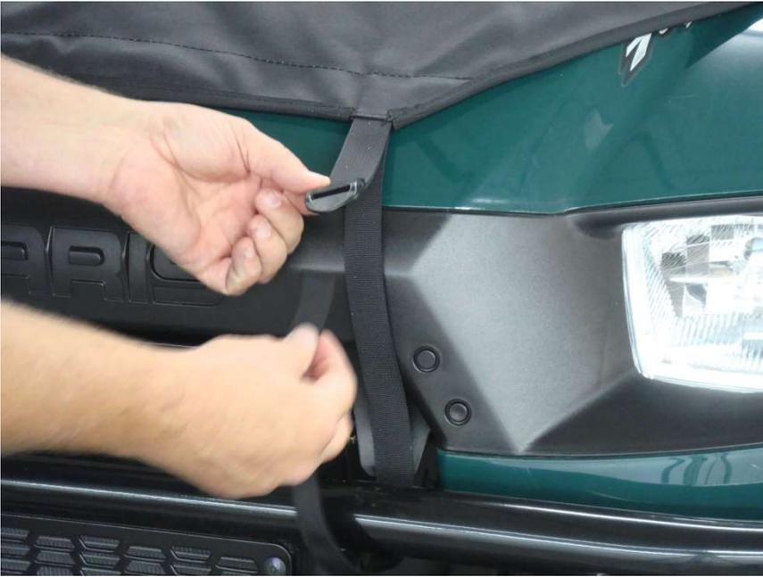
Figure 6.1 - run front hood straps around front bumper
