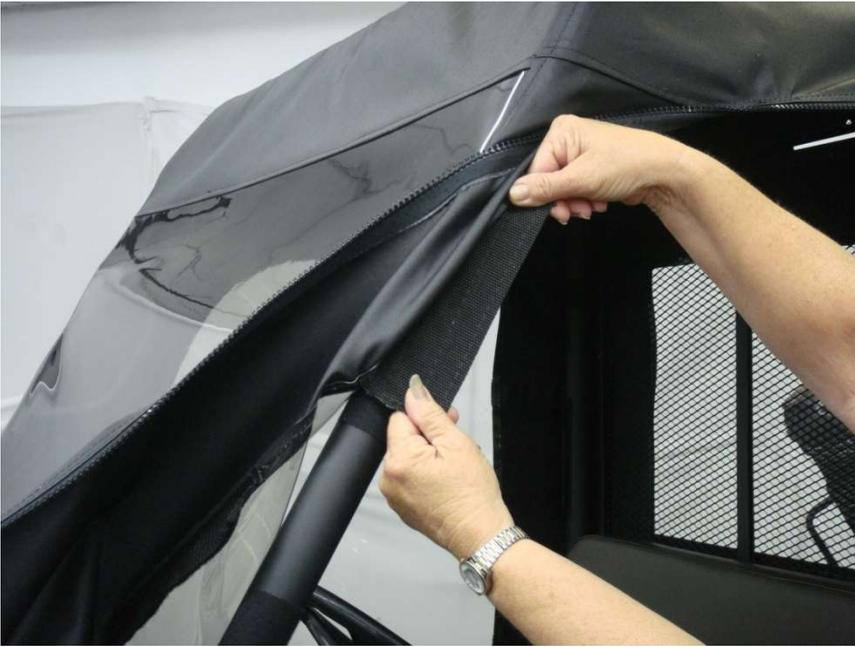
Figure 7.1 - attach top front Windshield roll bar 10" Velcro tabs
