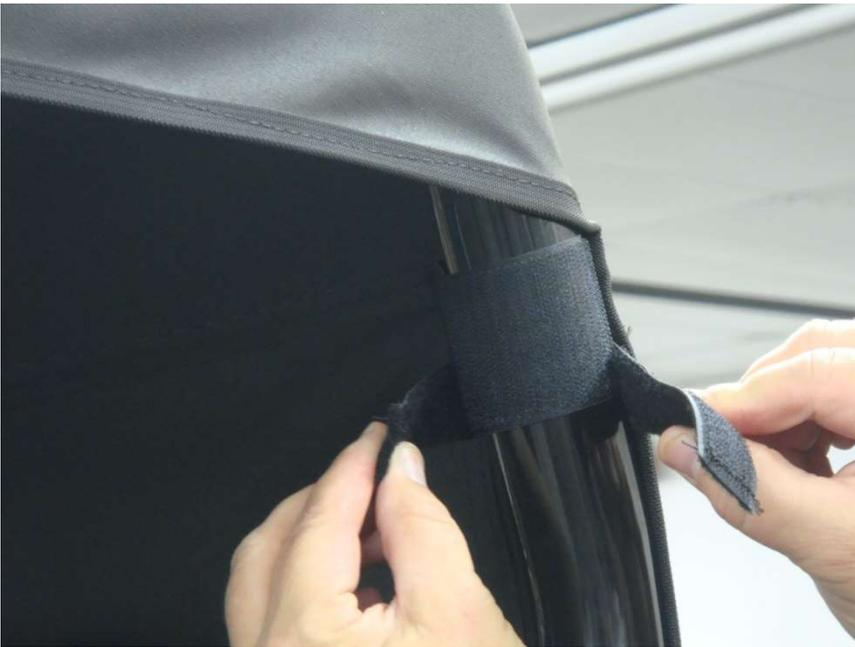
Figure 5.3 – attach rear Roll Bar upright top horizontal 6" Velcro Tabs
