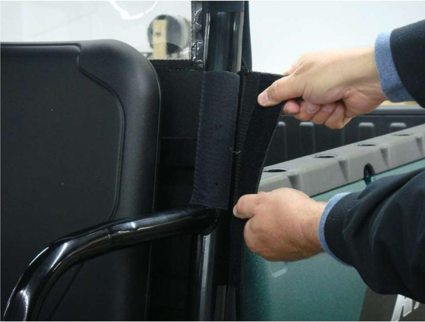
Figure 5.2 – attach rear middle roll bar upright 10" Velcro tabs
