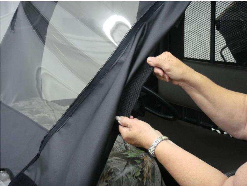
Figure 7.2 - attach middle front Windshield roll bar 10" Velcro tabs
