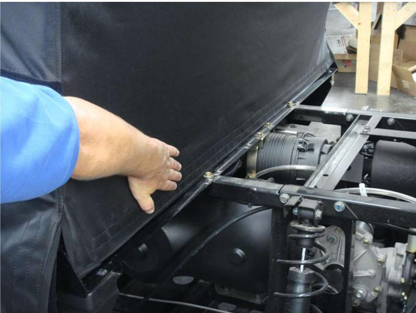
Figure 5.1 - square rear of enclosure to cab and attach rear enclosure Velcro tab to installed Velcro strip
