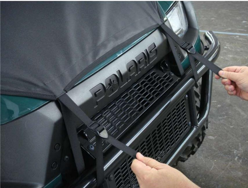
Figure 8.1 – Fully tighten both Hood Straps pulling downward on both at the same time
