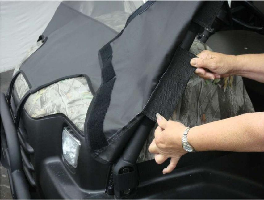
Figure 7.3 - attach bottom front Windshield roll bar 5" Velcro tabs
