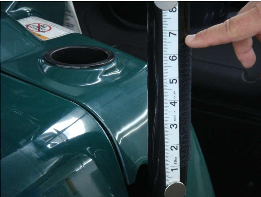
Figure 3.1 - attach 5" Velcro strips vertically approx 6 ½" above the front roll bar post cowl opening
