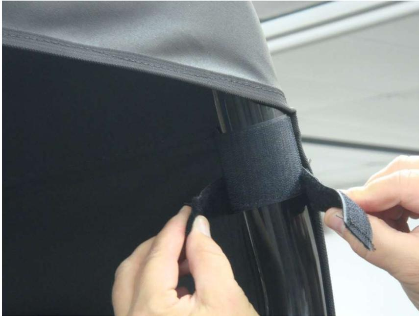
Figure 4.1 – attach rear Roll Bar upright top horizontal 6" Velcro Tabs
