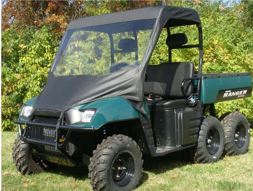
Figure 8.1 – Repeat all Steps until the enclosure fits snug to the vehicle roll bar cab and windshield is tight
