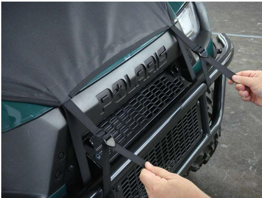
Fully tighten both Hood Straps pulling downward on both at the same time
