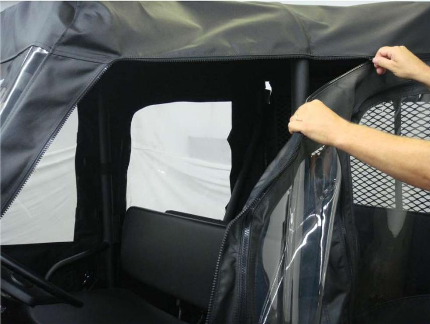
Figure 19.1 - Attach Side Door Panels by zipping them to the Top Cap
