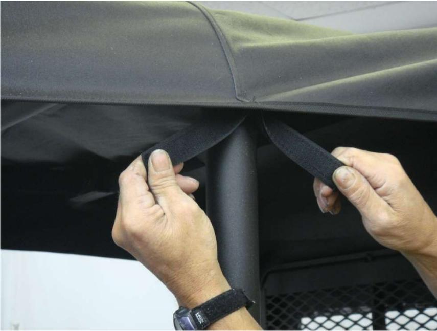
Figure 10.1 - attach Top Cap Center and Rear upper Velcro tabs to installed 6" Velcro Strips
