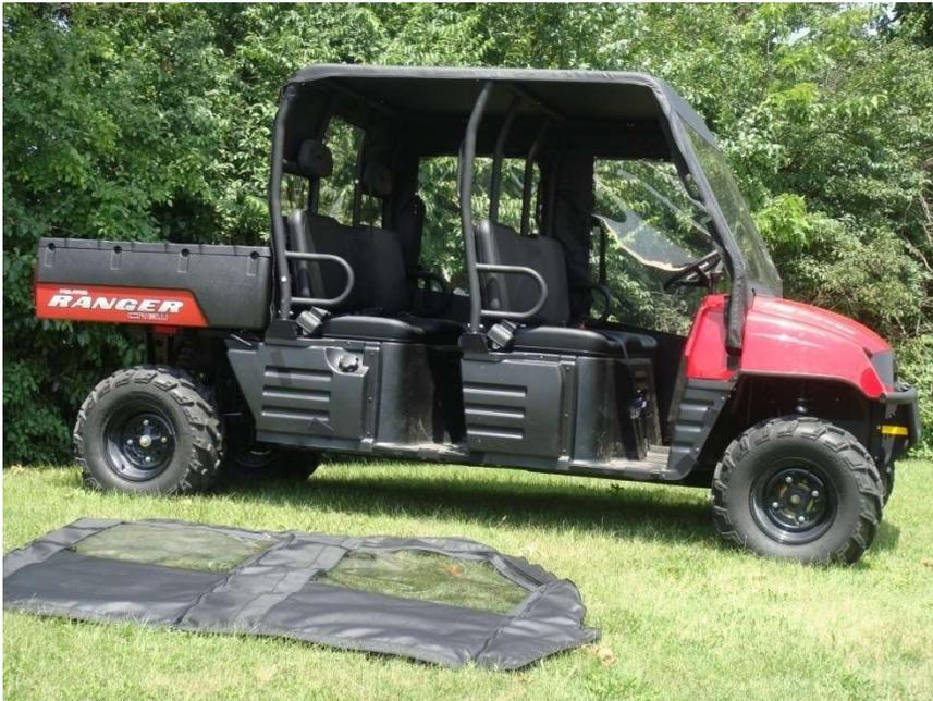
Figure 18.1 - Top Cap should fit snugly along the vehicle Top Roll Bar Structure
