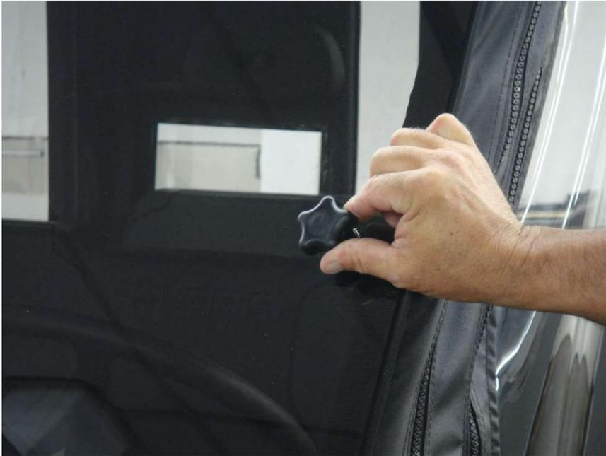
Figure 17.1 - Tighten Windshield Quick Connect Knobs
