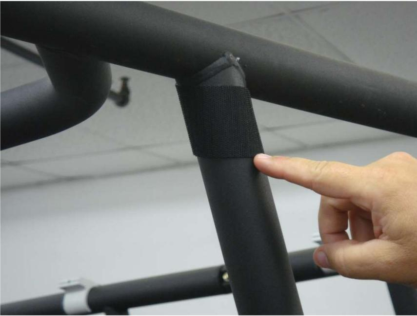
Figure 4.1 - install 6" Velcro Strips horizontally around Center Roll Bar uprights
