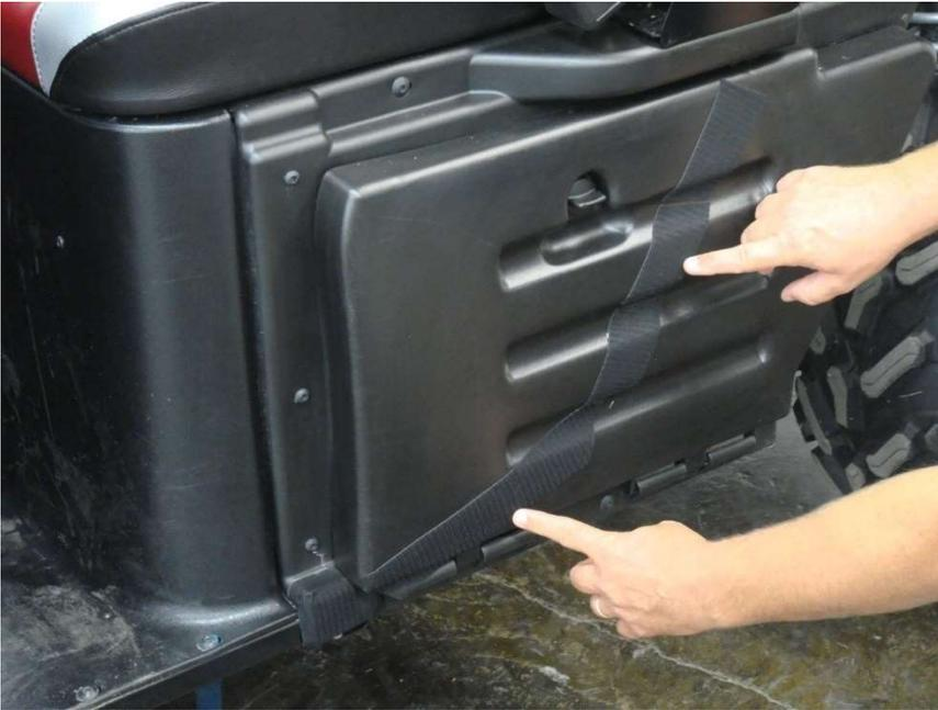
Figure 8.1 - Install 19.5" and 10" Velcro Strips on the Rear Door Side Panel
