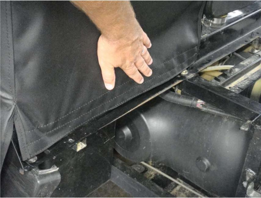
Figure 11.2 – Square Enclosure to Rear of Cab Frame and press Enclosure Velcro Tab onto 59” installed Velcro Strip
