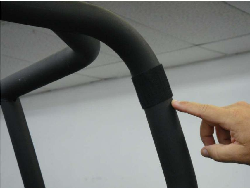
Figure 4.2 – install 6" Velcro strips horizontally around Rear Roll Bar Uprights
