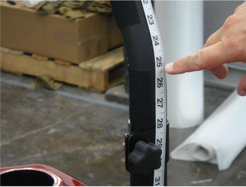
Figure 6.2 - install 12" Velcro strips along the inside edge of the front windshield Roll Bar upright lower section
