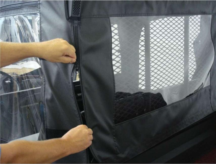
Figure 19.2 - attach Side Door Panels by Zipping them to the Rear Panel
