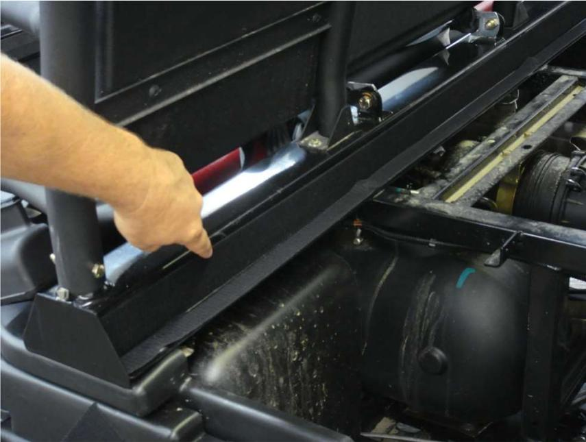
Figure 2.1 - attach 59" Velcro strip to Rear Cab Frame facing toward the rear of the vehicle
