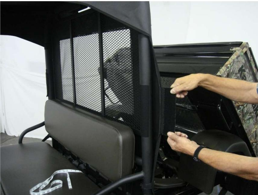
Figure 11.3 – attach 8” Rear Panel Roll Bar upright tabs to installed Velcro Strips
