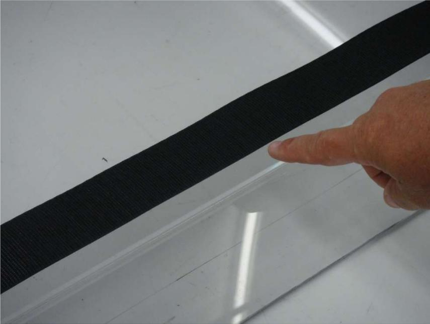
Figure 16.1 - Install the 60" Polycarbonate Windshield Velcro Strip below the Top Windshield Flap Bend
