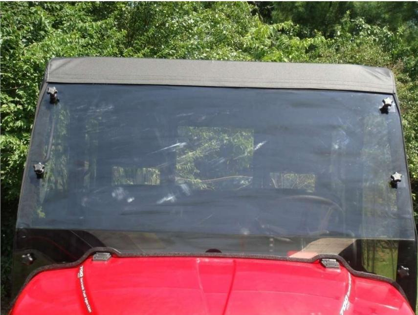
Figure 16.2 - Leading Windshield edge of enclosure should extend  $\frac{1}{4}$ " over the installed Windshield Velcro Strip so it is completely hidden.
