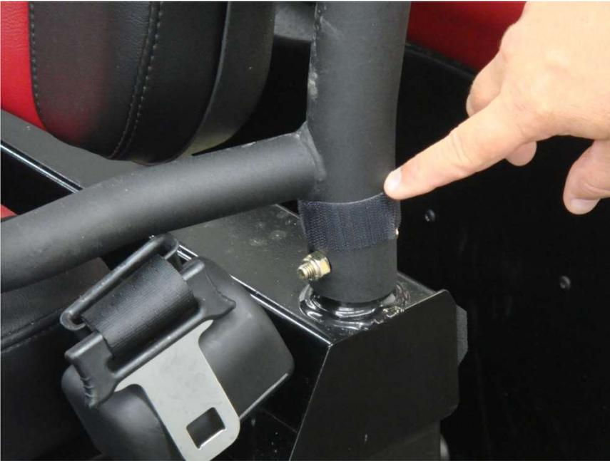
Figure 5.1 - install 6" (1" wide) Velcro strips horizontally around the bottom of the Center Roll Bar Uprights
