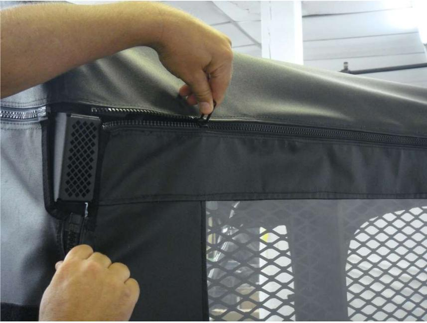
Figure 12.1 - attach Rear Panel onto Top Cap panel by Zipping the panels together
