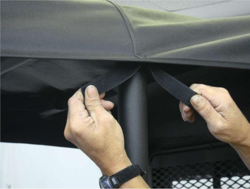
Figure 11.1 - attach Top Cap Center and Rear upper Velcro tabs to installed 6" Velcro Strips
