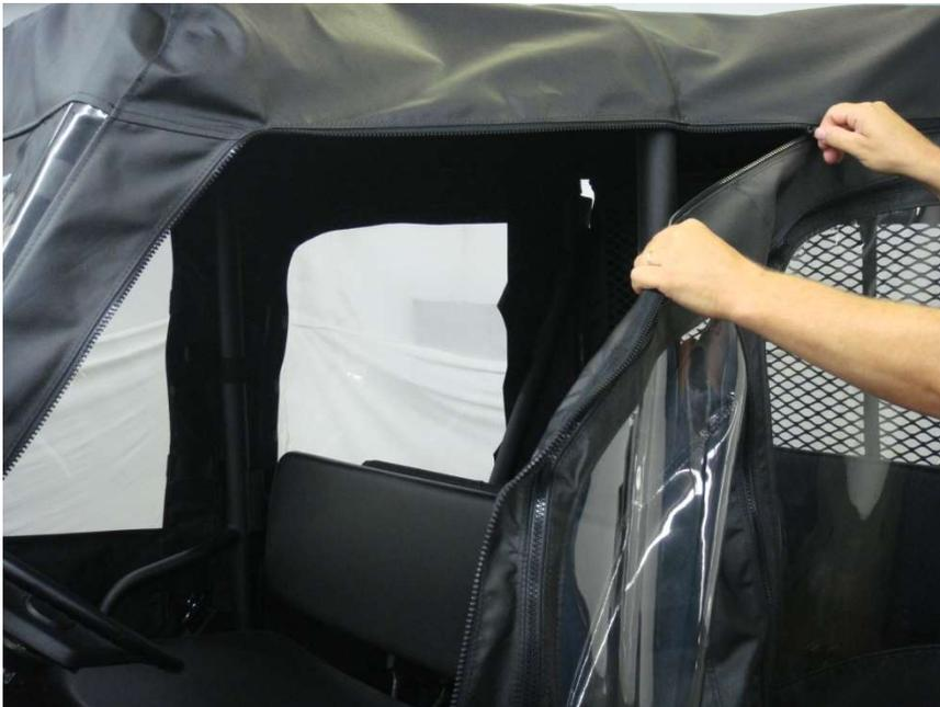
Figure 15.1 - Attach Side Door Panels by zipping them to the Top Cap
