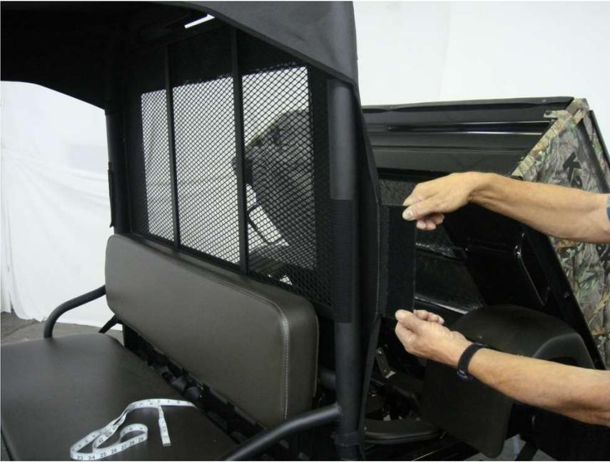
Figure 12.3 – attach 8” Rear Panel Roll Bar upright tabs to installed Velcro Strips
