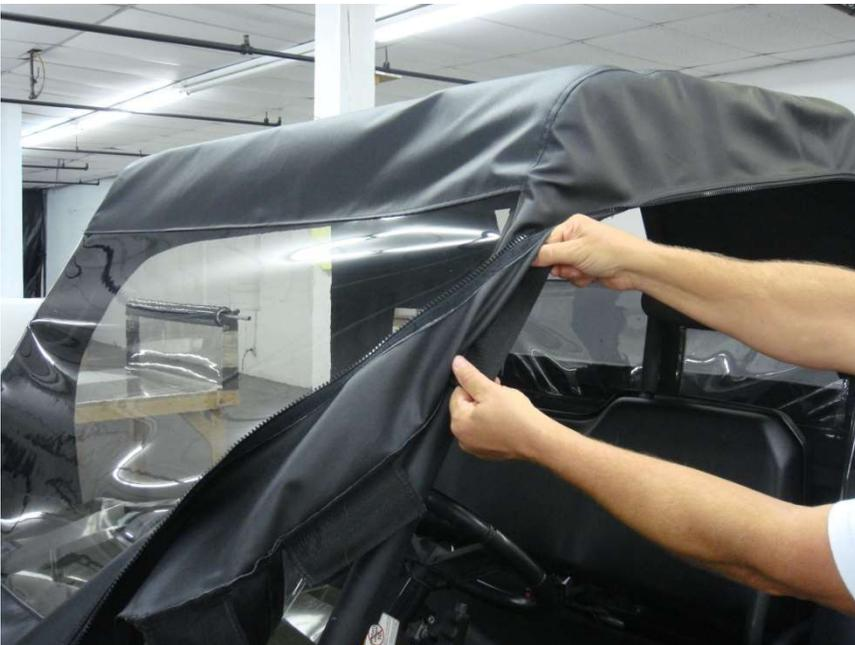
Figure 13.1 – attach Top and Middle 10” and Bottom 5” Windshield Velcro Tabs
