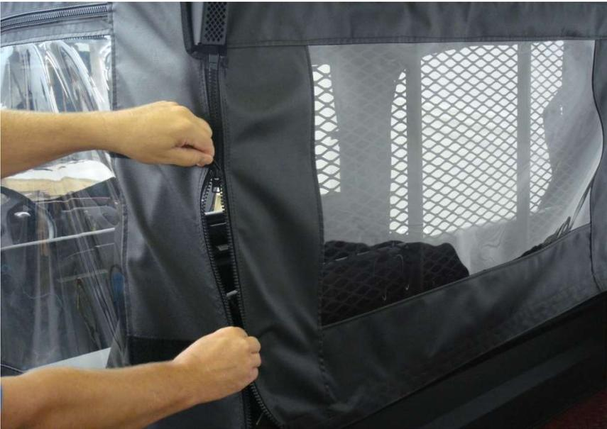
Figure 15.2 - attach Side Door Panels by Zipping them to the Rear Panel
