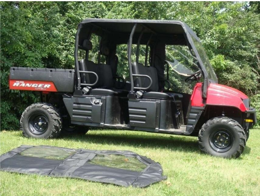
Figure 14.1 - Top Cap should fit snugly along the vehicle Top Roll Bar Structure
