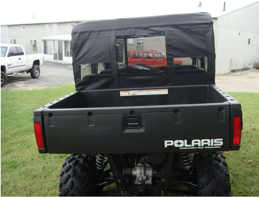
Figure 14.2 – Rear Panel should fit tightly across the back of the vehicle
