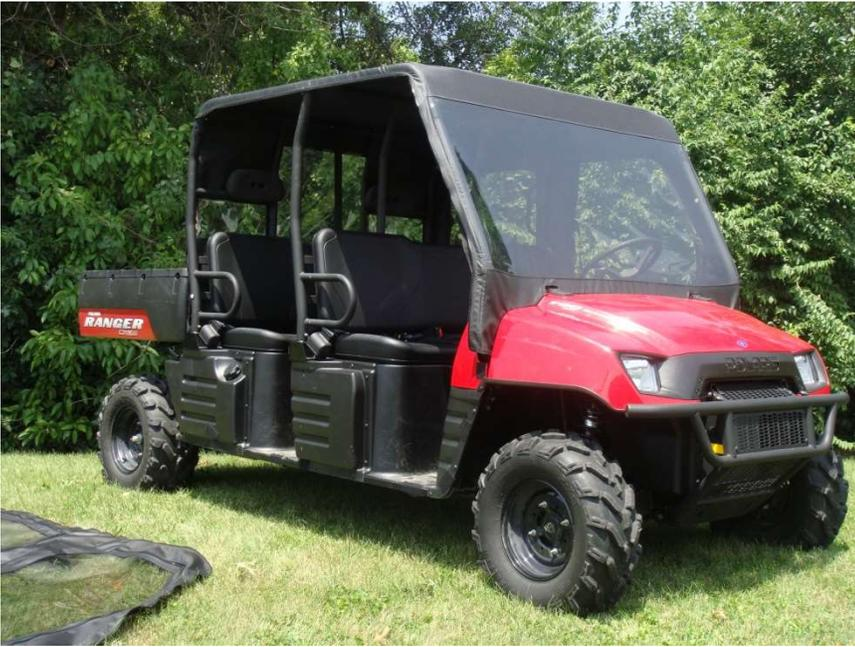
Figure 13.2 – Windshield should be tight at this step of the installation
