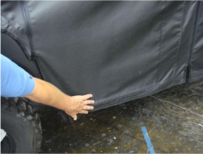
Figure 16.1 - Press Side Door Velcro Tabs onto installed Side Door Velcro Strips
