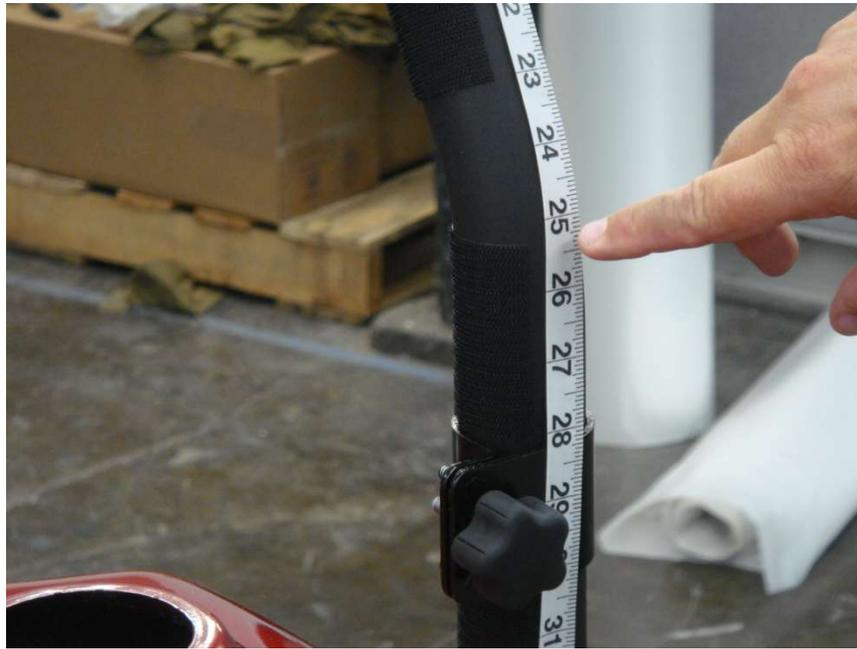
Figure 8.2 - install 12" Velcro strips along the inside edge of the front windshield Roll Bar upright lower section
