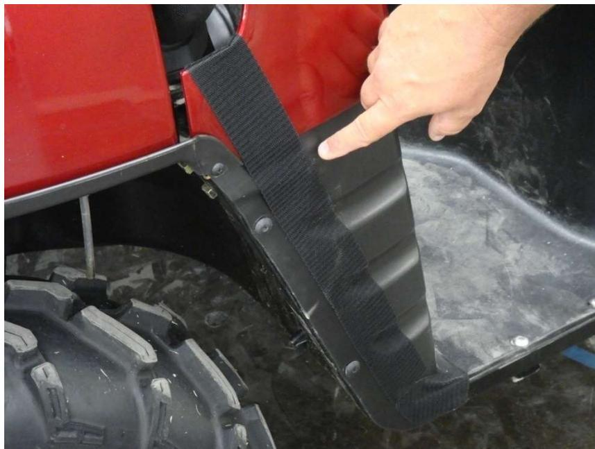
Figure 9.1 – attach 19" Velcro strips Vertically to the lower section of the Dash Cowl side panel and 4" strips horizontally at the bottom
