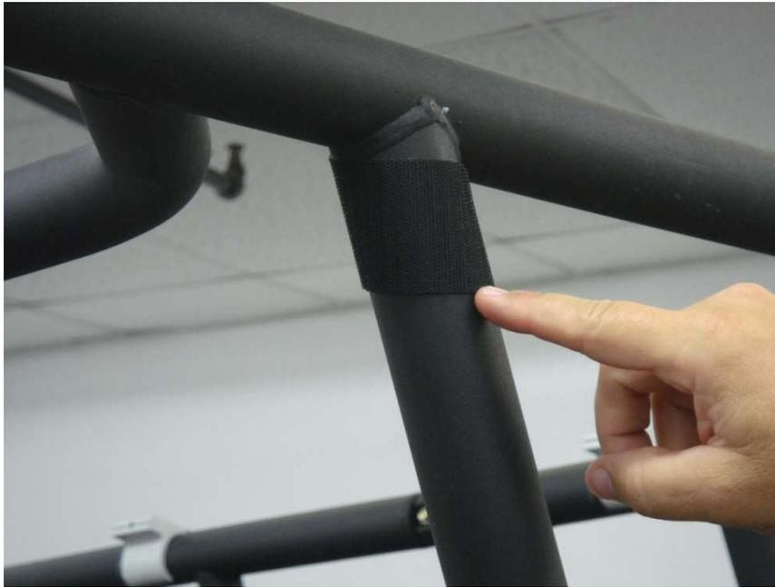
Figure 6.1 - install 6" Velcro Strips horizontally around Center Roll Bar uprights
