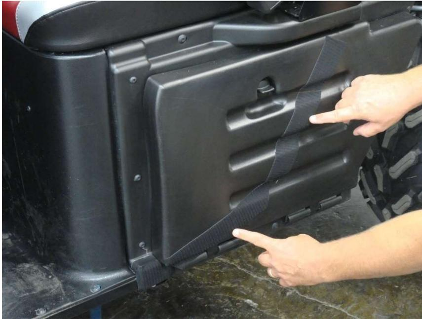
Figure 10.1 - Install 19.5" and 10" Velcro Strips on the Rear Door Side Panel
