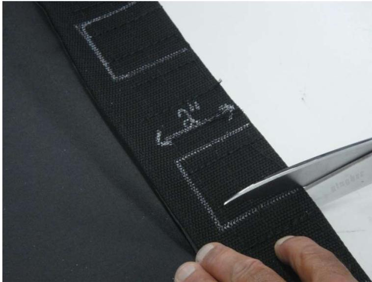
Figure 16.1 - Cut out Velcro Tab Binding at each Clamp Location
