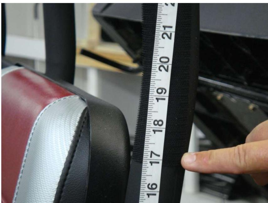
Figure 5.1 attach 8" Velcro strips vertically on the Rear Roll Bar uprights
