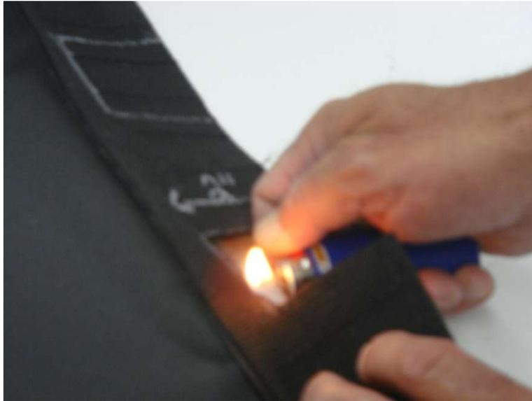
Figure 16.3 - With a lighter briefly melt the frayed ends of the fabric to prevent future fraying of the material
