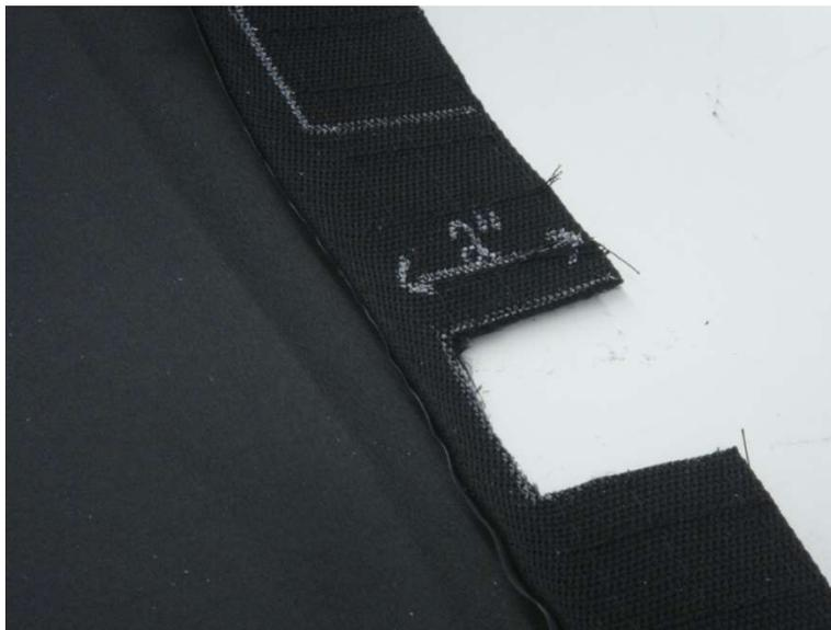
Figure 16.2 - DO NOT CUT VELCRO TAB BINDING STITCHES ATTACHING BINDING TO THE ENCLOSURE – stay back at least 1/2" from Stitching while Cutting
