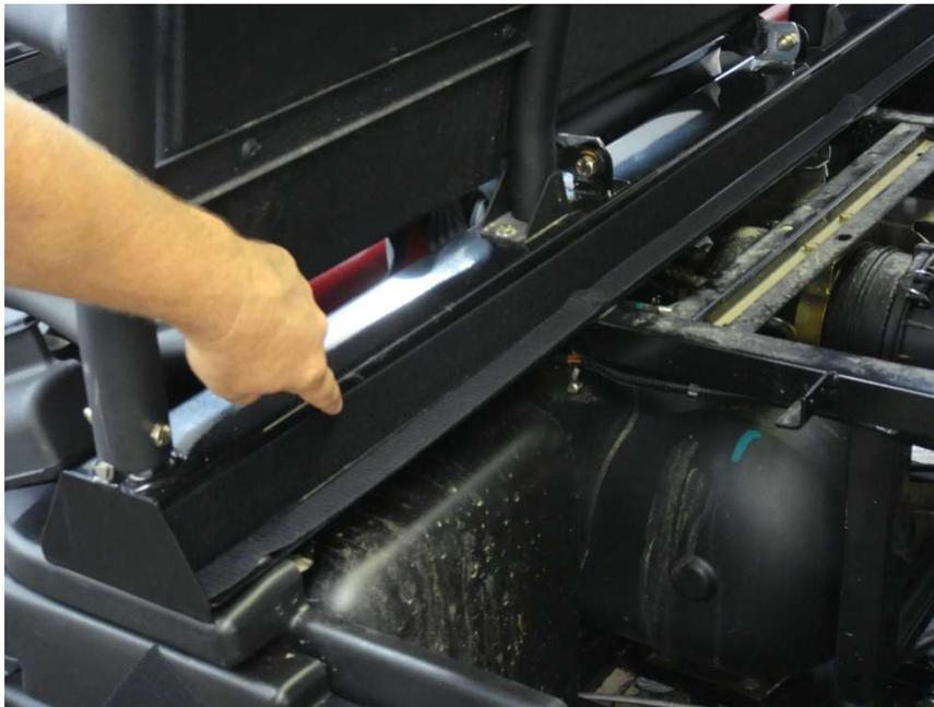
Figure 4.1 - attach 59" Velcro strip to Rear Cab Frame facing toward the rear of the vehicle
