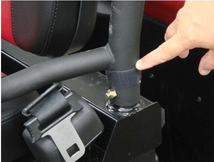
Figure 7.1 - install 6" (1" wide) Velcro strips horizontally around the bottom of the Center Roll Bar Uprights
