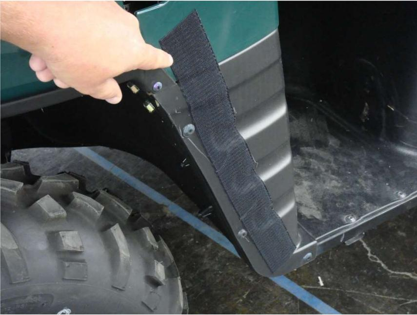
Figure 4.1 – attach 18 ½” Velcro Strips vertically along the lower Front Cowl Panel
