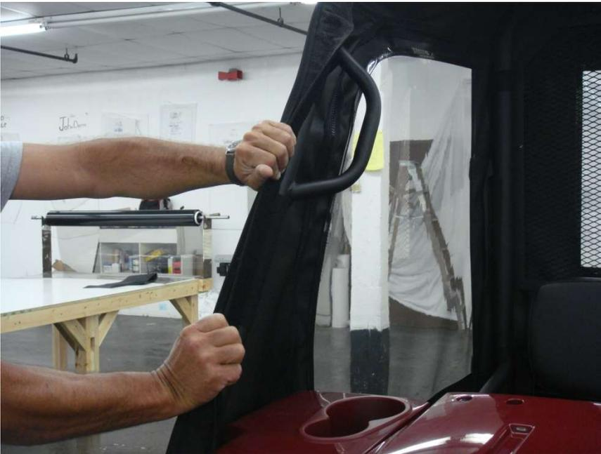
Figure 10.1 – attach Windshield Roll Bar post Velcro Tabs to installed 24", 11" and 6" Velcro Strips
