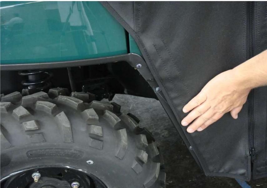
Figure 11.3 – attach Door Front Cowl Panel Enclosure 18 ½" Velcro Tabs
