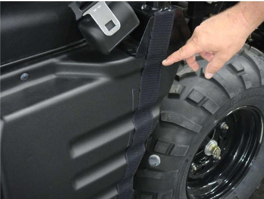
Figure 3.1 - attach 20" Velcro Strips vertically along the lower Rear Door Panel
