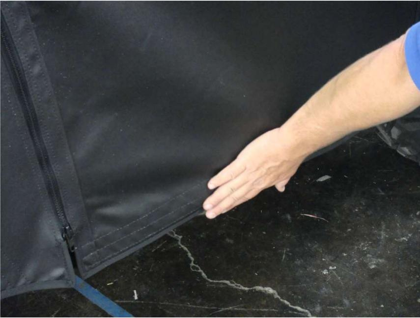
Figure 11.2 – attach Door Rocker Panel Enclosure 27" Velcro Tabs
