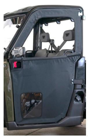
**21.** Move the door into the "closed" position. With the window down, you can access the striker plate from the outside of the vehicle to make adjustments easier.
