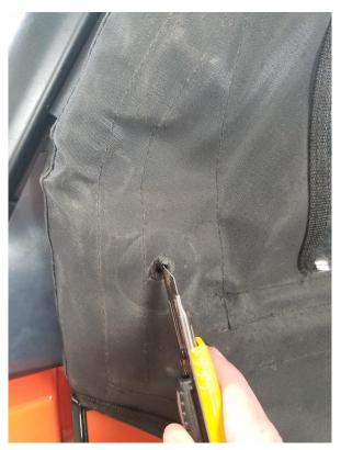
**35.** Using a sharp razor or utility knife, cut the textile so the mirror mounting bolt can pass through.
