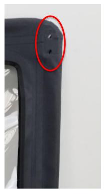
17. Holes need to be cut in door textile panels in order to mount the Upper and Lower Sliding Hinges. Ensure textiles are tight and fit as desired before marking and cutting holes. Take a sharp scribing tool and punch a small hole through the textile indicating the center of the slot. Take a razor blade and carefully cut out the small amount of textile so that the supplied M8 bolt may pass through the plate and the textile. Repeat this process for the lower mounting location.
