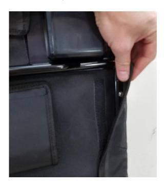
**12.** Continuing down the door, attach long flap at the forward section of the lower door tubing to the hook Velcro on the inside of the panel.
