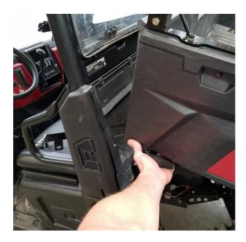
**2.** To install Lower Hinge Plate begin by moving the bed into the dump position. This is done in order to access the factory Torx head fasteners
