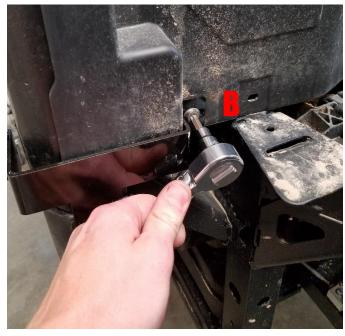
**4.** Install Lower Hinge Plate using factory Torx Head fasteners. (Body plastics may move when fasteners are removed. Be sure to realign holes to ensure the fasteners line up with the threaded holes in the sheet metal behind the plastics.)
