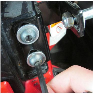
**31.** With the striker bolt in the correct location, fully tighten down the striker bolt to the striker plate and fully tighten the plate to the ROPS Structure.
