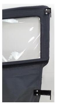
**18.** Pass M8x25mm bolts through the Upper Sliding Hinge, textile, then the welded on door plate. Attach using M8 washers and lock nuts as shown. Repeat steps for Lower Sliding Hinge using M8x25mm bolts, M8 washers and lock nuts. Do not fully tighten at this time. Sliding Hinges are slotted for door adjustment.
