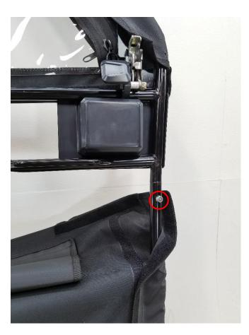
**9.** Attach Upper and Lower door frames using M6x25mm button head fasteners and corresponding M6 locknuts. The locknut should be on the inside of the door frame as shown.
