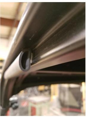
**19.** Clean the highlighted area of the ROPS structure and bodywork with rubbing alcohol or window cleaner. **(Failure to clean ROPS structure and bodywork will result in gasket falling off and doors not sealing properly!) Adhere the provided gasket into the outer channel of the roll cage as shown by the highlighted area above. Be sure the gasket is oriented the same as the image above.**
