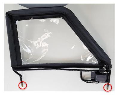
**1.** Locate attachment locations circled on both the Lower and Upper Door Frames. The sleeve tubing in the Upper door frame will slide into the tubing of the lower door frame.
