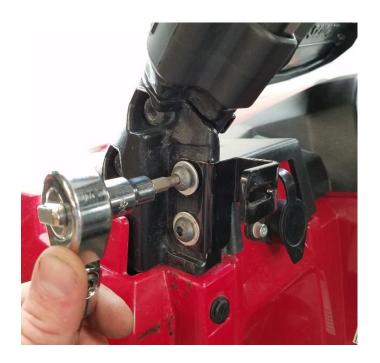
**5.** Move to the front corner of the ROPS structure. The Striker Plate will be installed using M8x20mm fasteners and M8 Washers in the holes provided on the ROPS structure as shown. (note these holes are slotted for striker adjustment. Do not fully tighten at this point.)
