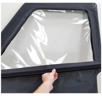
**15.** Pull Upper door textile down firmly and attach to loop Velcro located on the outside of the lower panel as shown.
