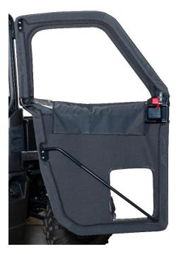
20. Insert the Sliding Hinge Pins into the Hinge Mount Barrels and roll down the window for easier adjustment.
