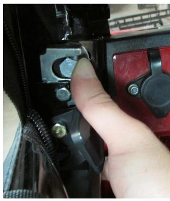
**23.** With the striker bolt loose and door pressed firmly against the body work and gasket, move the striker bolt into the closed position of the rotary latch. There should be two clicks when it is fully latched. Note the location of the striker bolt on the striker plate. This will give you a good starting point for adjusting the door.
