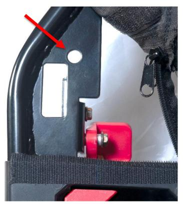
**34.** Locate the mirror mounting bracket on the inside of the door frame. Mark the location of the hole with a punch so that it can be seen on the outside of the door textile.
