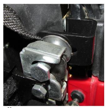
**30.** The door should be adjusted in the forward/rearward direction so that the striker bolt head does not contact the latch. The image above shows the correct positioning of the striker bolt.
