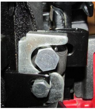
**28.** Shown above is the correct alignment for the striker bolt and latch when the door is fully closed.
