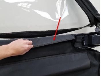
**10.** Pull upper rear flap from lower door panel snugly over the door arm bar and secure flap to hook Velcro.
