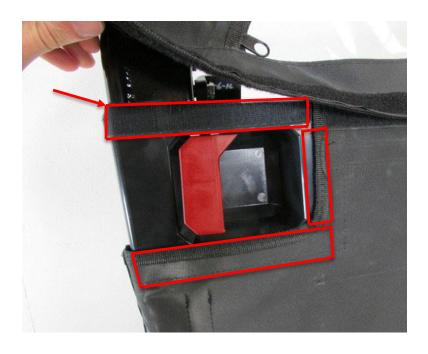
**14.** Cut and place pieces of 1" wide adhesive hook Velcro onto plastic molded pocket in the areas outlined. This will keep the upper door textile secure at the front of the door.
