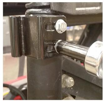
**1.** Install Upper Hinge Plate and Upper Backing Plate onto the mounting location at the upper rearward part of the ROPS structure. Install using M8x20mm fasteners and M8 Washers as shown. Do not fully tighten at this point as adjustments will need to be made when hanging the door structure.
