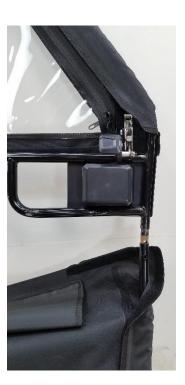
**8.** Align Door frames, ensuring the two pieces are the same side (Both Driver sides, or both Passenger sides. Driver Door shown) and join the two door halves together. It will help to detach some of the Velcro on the lower door frame in order to make access to the tubing easier.
