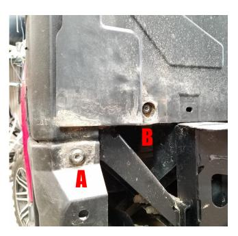
**3.** Locate the factory Torx head fasteners at positions "A" and "B". These will be used to attach the Lower Hinge Plate. Remove fasteners.
