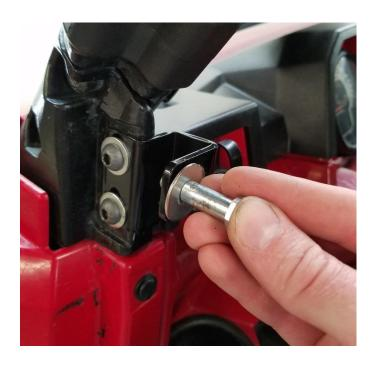
**6.** Attach striker bolt in the remaining slot on the Striker Plate in the orientation shown. Install with supplied nut. (This will adjust how far in and out the door is from the front of the body) (Do not fully tighten at this point.)
