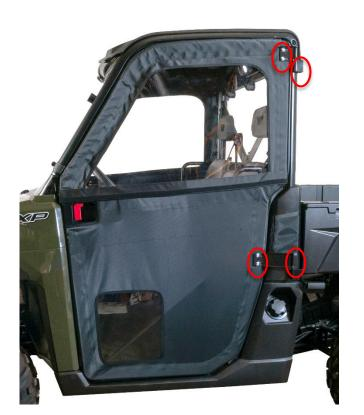
**33.** Once the door has been adjusted as desired, fully tighten down all fasteners on door hinge sliding plates, and hinge mounts. Before operation, ensure all Velcro is securely fastened.
