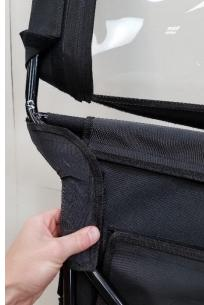
**13.** At the rear of the lower door panel, wrap upper flap tightly around tubing to hook Velcro on the inside of the panel in the area shown.
