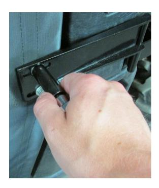
**25.** Move the door back into the closed position, again pressed firmly against the gasket on the bodywork. This may require you to move the striker assembly up or down in order for the latch to fully engage. At this point tighten the door plate bolts just enough to keep the door from sliding forward and back.
