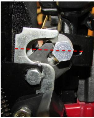
**27.** Shown above is the correct alignment for the striker bolt and latch just before the door is closed. The bolt should line up in the center of the relief in the latch. This will allow the door to close smoothly.
