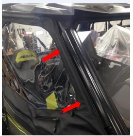
TIP: The OEM door may need to be adjusted forward and backward to create a seal on the ROPS, ensure the front triangle creates a good seal.
