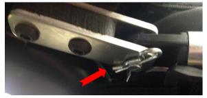
10) Align Brackets on Door Frame to holes on the lower door.
