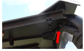
Remove outer plastic panel from the inside of the door by removing 6 screws (see photo next column)
